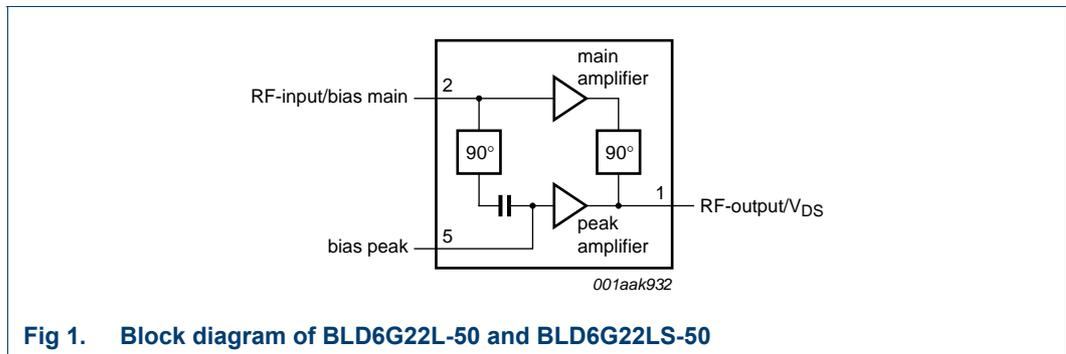
Fig 1. Block diagram of BLD6G22L-50 and BLD6G22LS-50
