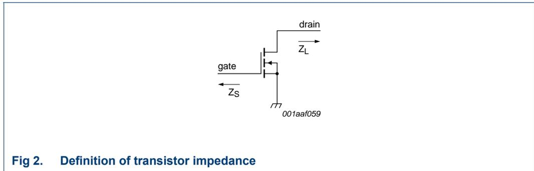
Fig 2. Definition of transistor impedance
