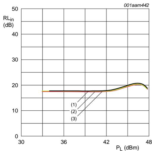
$V_{DS} = 28\text{ V}$ ;  $I_{Dq} = 170\text{ mA (main)}$ ;  $T_{case} = 25\text{ }^\circ\text{C}$ ;  $V_{GS(amp)peak} = 0\text{ V}$ ;  $\delta = 10\%$ ;  $t_p = 100\text{ }\mu\text{s}$  on 1 ms period.
