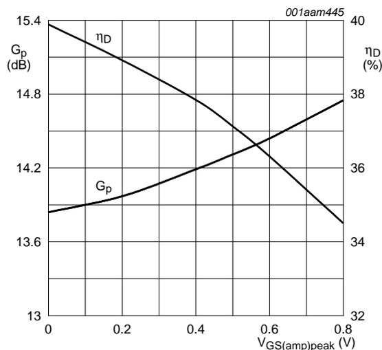
$V_{DS} = 28\text{ V}$ ;  $I_{Dq} = 170\text{ mA}$  (main);  $T_{case} = 25\text{ }^{\circ}\text{C}$ ;  $f = 2140\text{ MHz}$ ; 2-carrier W-CDMA; PAR = 8.3 dB at 0.01 % probability on CCDF.
