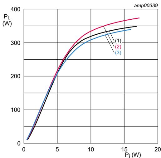
$V_{DS} = 28\text{ V}; I_{Dq} = 400\text{ mA}; t_p = 300\text{ }\mu\text{s}; \delta = 10\text{ }\%$ .
