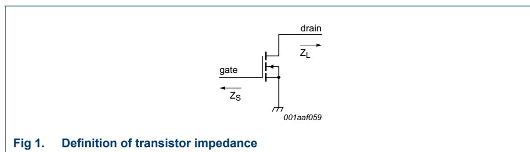
Fig 1. Definition of transistor impedance
