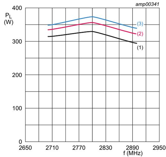
$V_{DS} = 28 \text{ V}$ ;  $I_{Dq} = 400 \text{ mA}$ ;  $t_p = 300 \text{ } \mu\text{s}$ ;  $\delta = 10 \text{ \%}$ .
