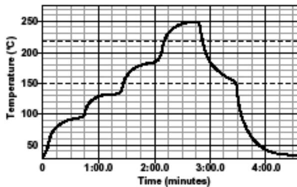
Figure 9. Lead-free (SnAgCu) Solder Ball Reflow Profile
