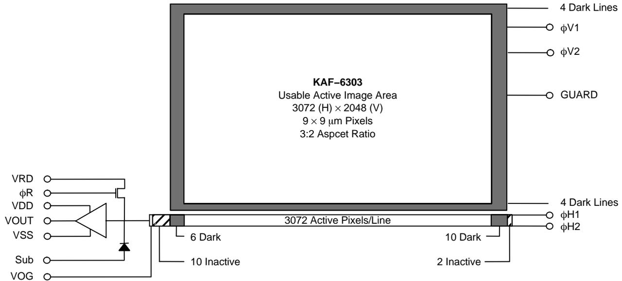
Figure 2. Block Diagram
