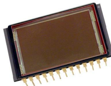
**Figure 1. KAF-6303 Full Frame CCD Image Sensor**
