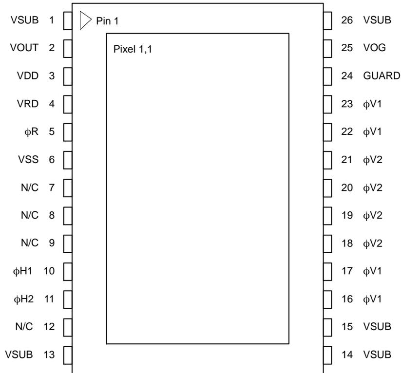
**Figure 4. Pinout Diagram**
