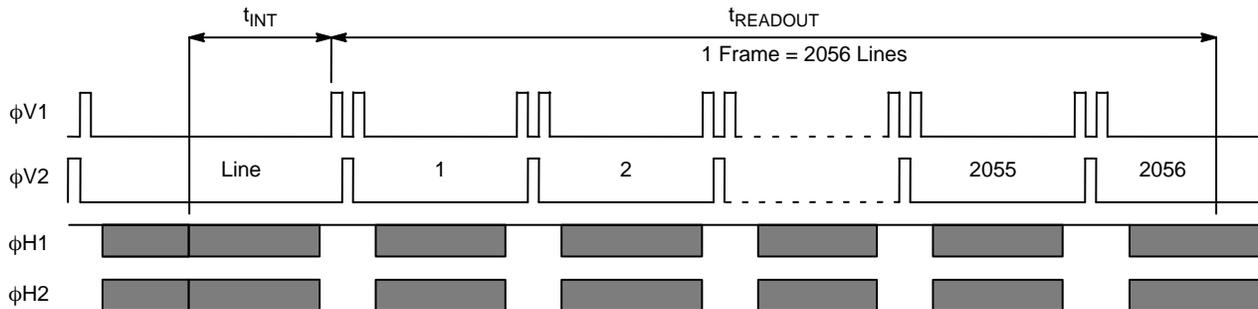
**Figure 7. Frame Timing**
