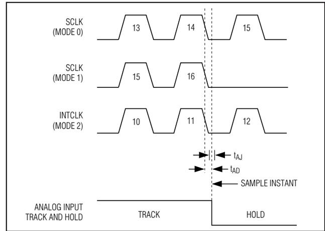
Figure 21. Aperture Diagram
