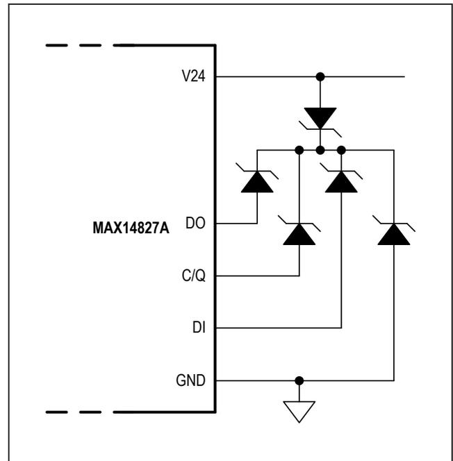
Figure 9. MAX14827A Operating Circuit with TVS Protection
