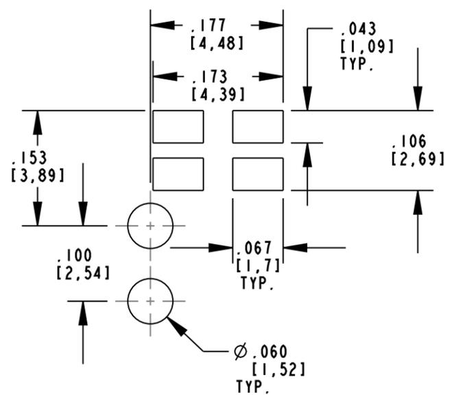
**RECOMMENDED SOLDER PAD LAYOUT & HOLE PATTERN GAUGE**
