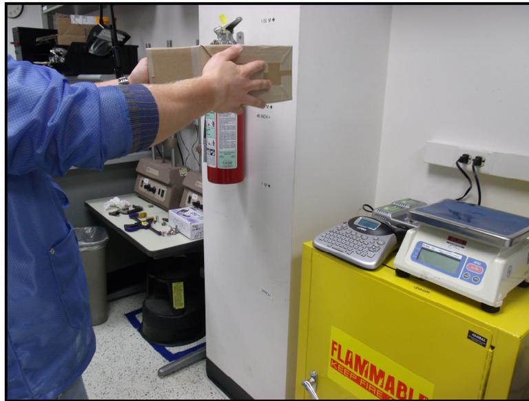
Figure 6 – Transit Drop Set Up
