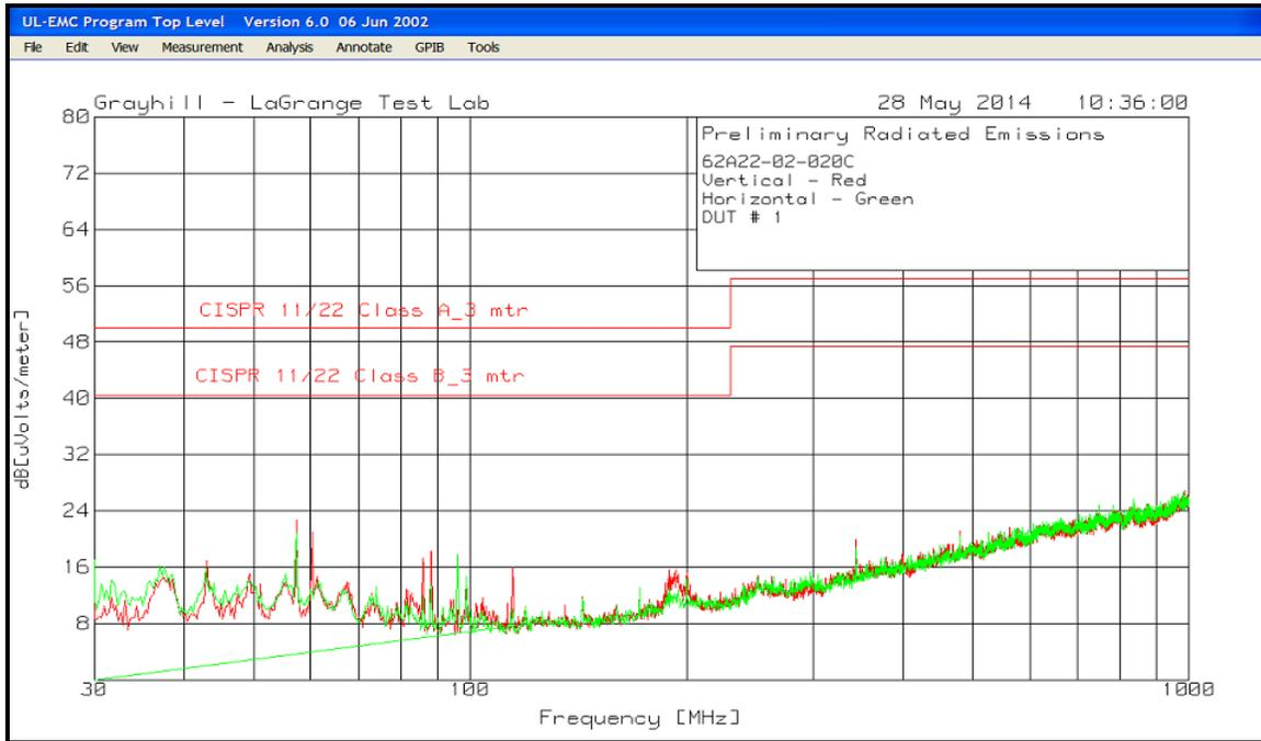
Figure 5 – Radiated Emissions Results (Red Vertical, Green Horizontal)
