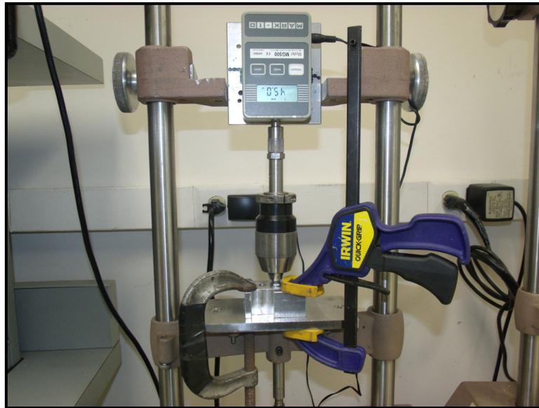
Figure 3– Pull Out Force Setup
