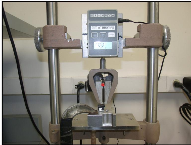
Figure 4– Cable Strength Setup
