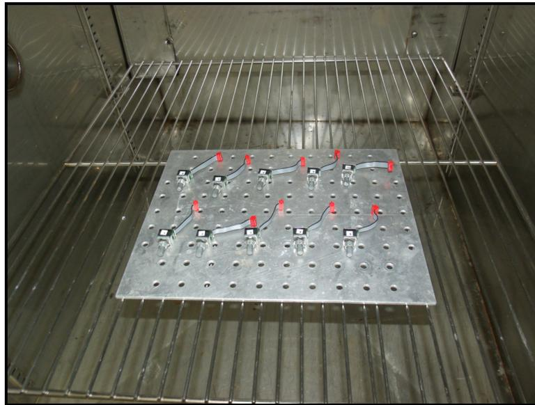
Figure 1 – Storage Low Temperature Test Setup
