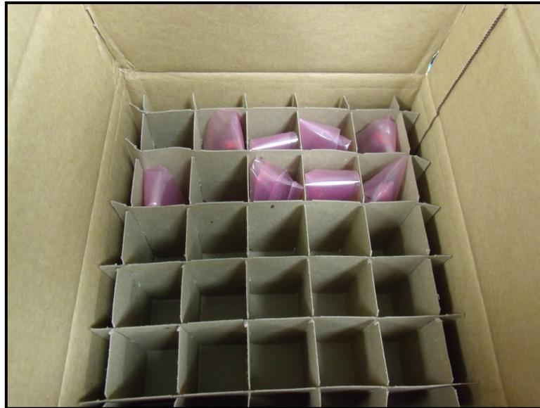
**Figure 8 – DUT Packaging after Transit Drop**
