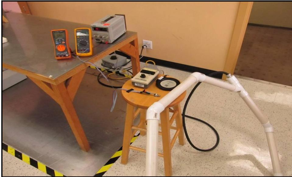
Figure 12 – Magnetic Field Test Setup
