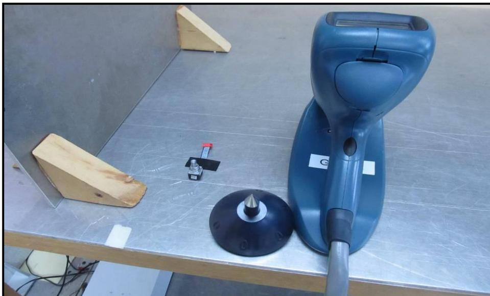
**Figure 10 – Electrostatic Discharge Test Setup (Un-Powered)**
