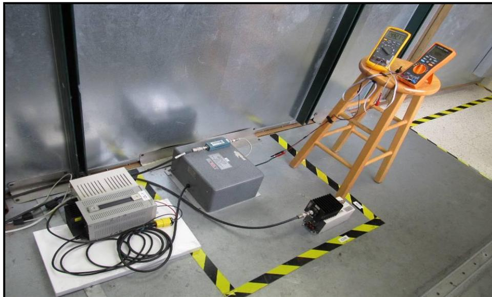
**Figure 7 - Conducted Emissions Test Setup**
