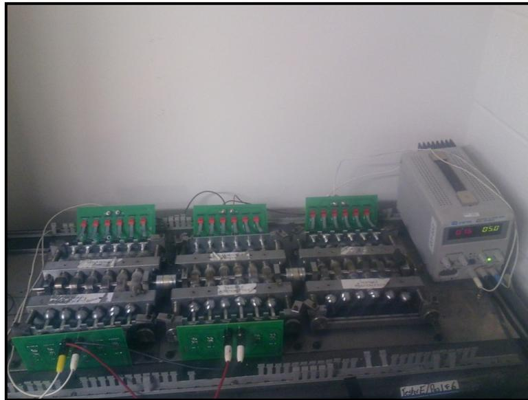
Figure 13 – Push Button Life Test Setup
