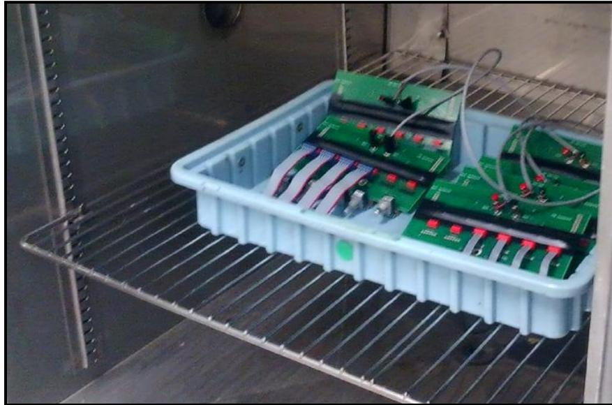
Figure 11 – Operating Low Temperature Test Setup
