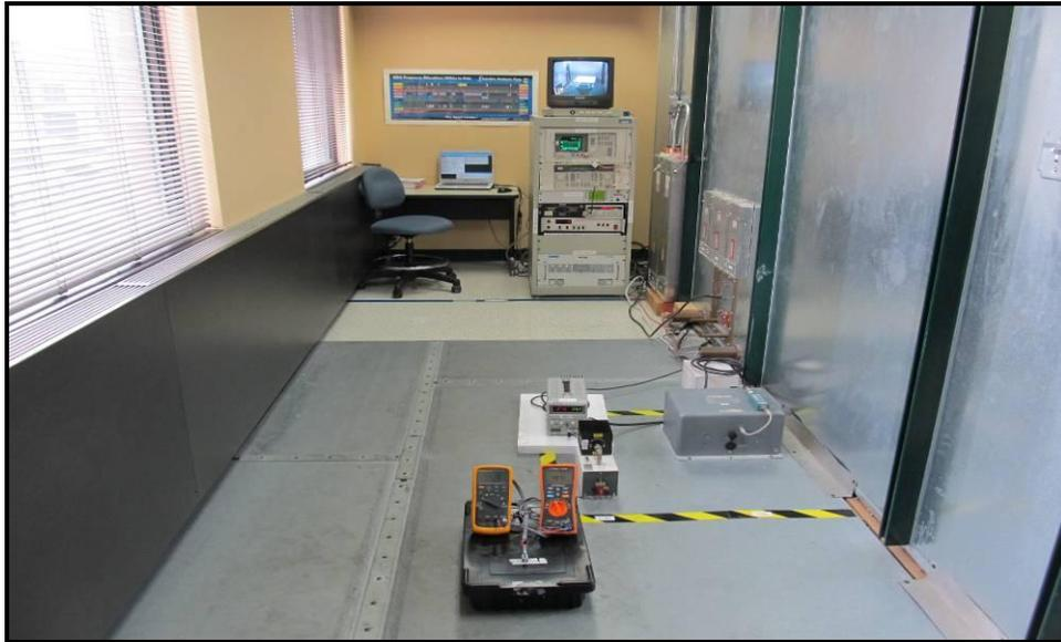
Figure 6 – Conducted Immunity test setup
