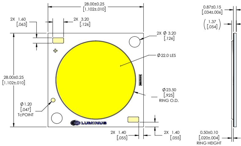
Note: Unless otherwise specified, tolerance is  $\pm 0.3\text{mm}$
