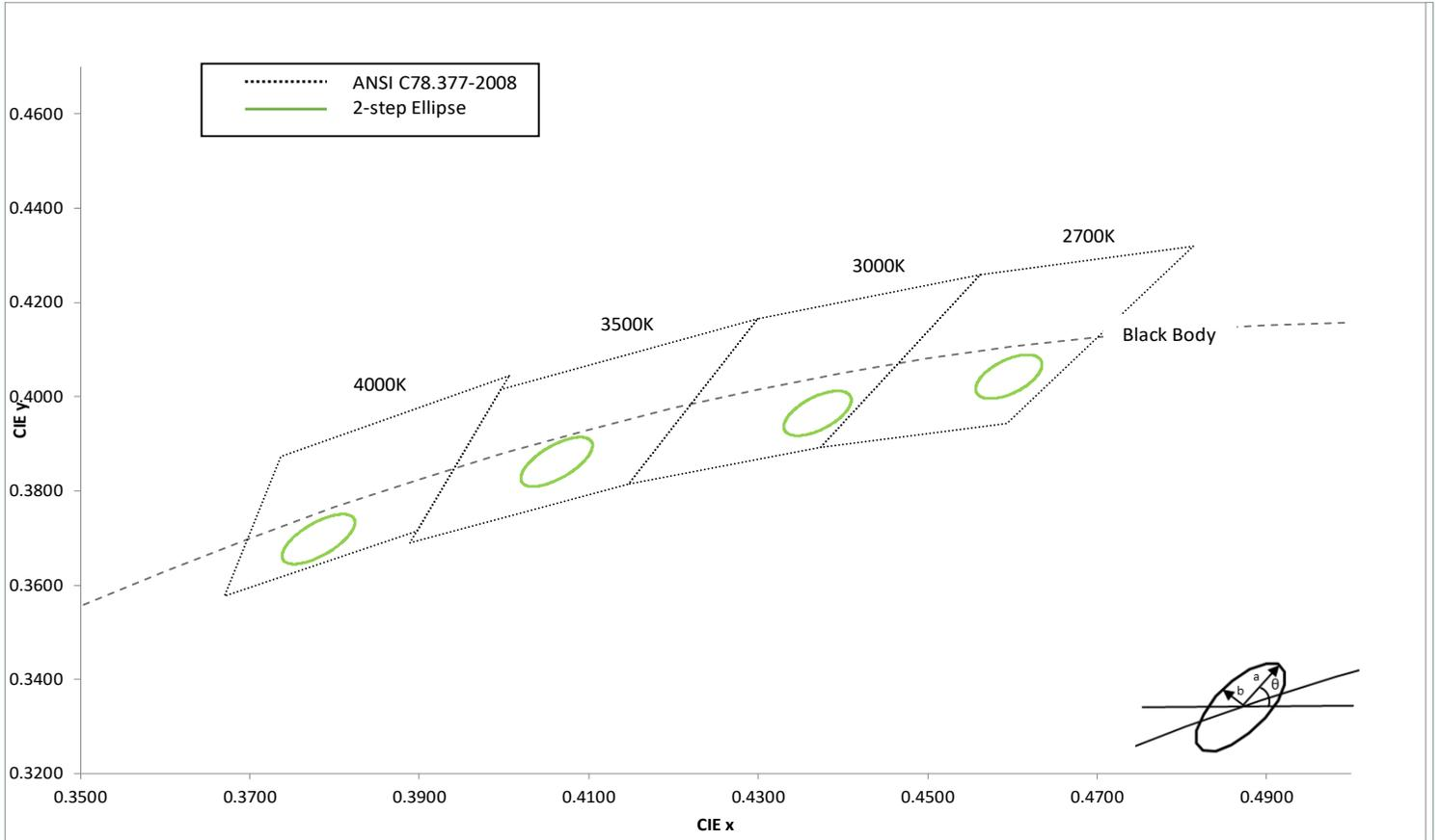
The following tables describe the chromaticity bin center points, the orientation angle for the MacAdam ellipse ( $\theta^\circ$ ), and the maximum radii for the ellipses. The ANSI Bin is provided for reference.
