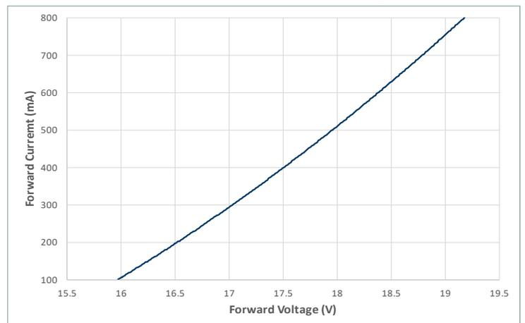
**CXM-4 Optical & Electrical Characteristics - 18V**
