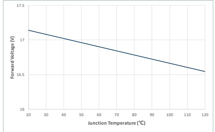
**CXM-6 Optical & Electrical Characteristics - 36V**
