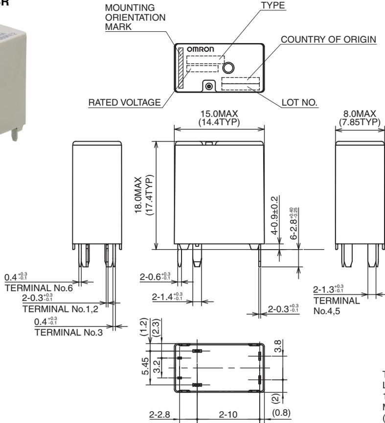
FOR REFERENCE : PCB MOUNTING HOLES (BOTTOM VIEW)
