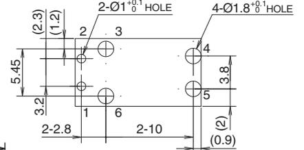
\*Please study & choose other appropriate hole diameters if confirmed the diameter values recommended above don't work with the soldering process.
