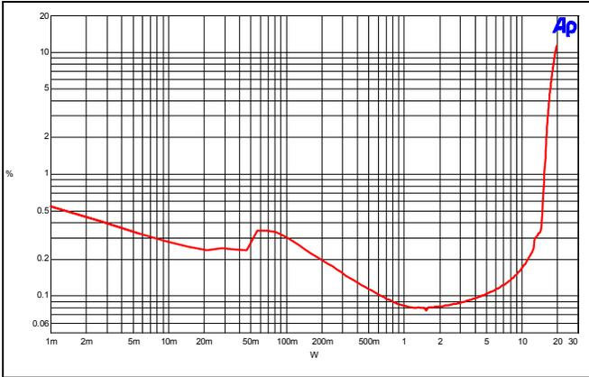
THD+N vs. Output Power ( $R_L = 8\Omega$ , SE)
