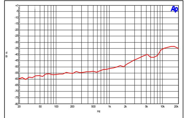
PSRR vs. Frequency ( $R_L = 8\Omega$ , BTL)
