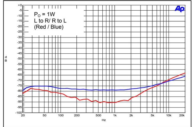
PSRR vs. Frequency ( $R_L = 4\Omega$ , SE)
