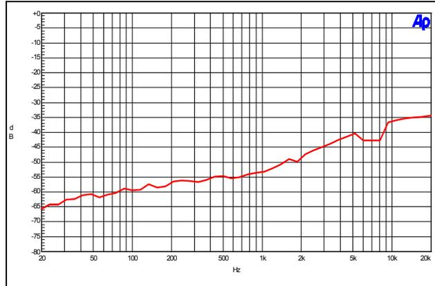
PSRR vs. Frequency ( $R_L = 8\Omega$ , SE)
