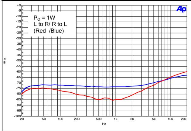
Crosstalk vs. Frequency ( $R_L = 8\Omega$ , SE)
