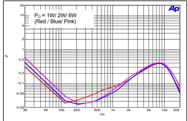
THD+N vs. Output Power ( $R_L = 8\Omega$ , BTL)
