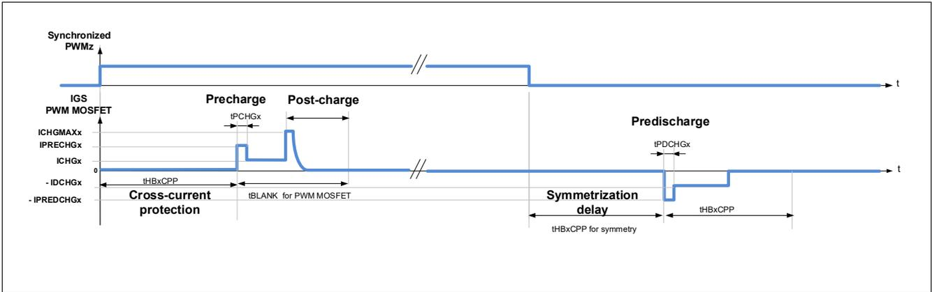
Figure 15 PWM overview showing pre-charge, pre-discharge and post charge phases, AGC[1:0] = 10<sub>B</sub> or 11<sub>B</sub>, POCHGDIS = 1<sub>B</sub>.
