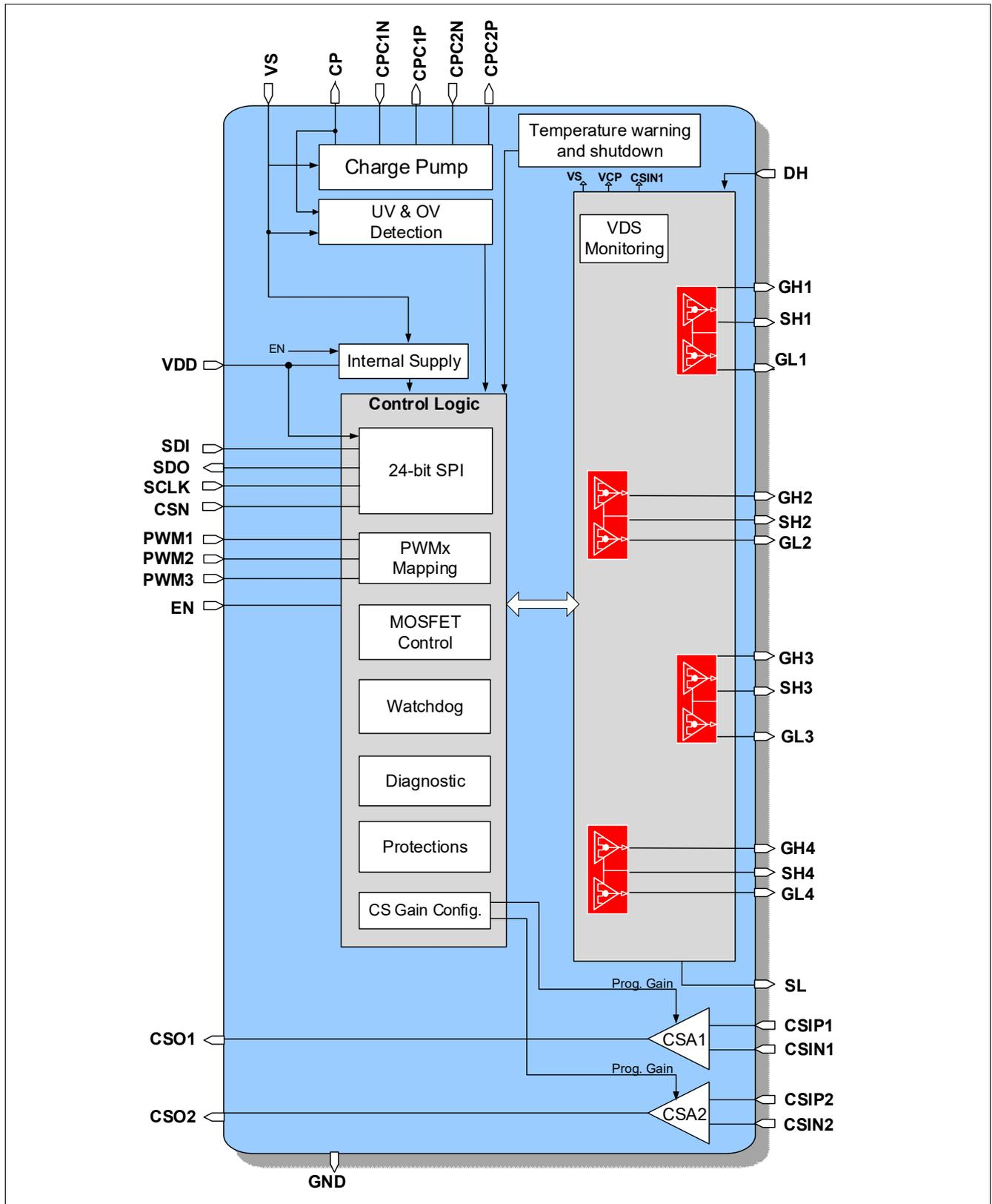
Figure 1 Block diagram
