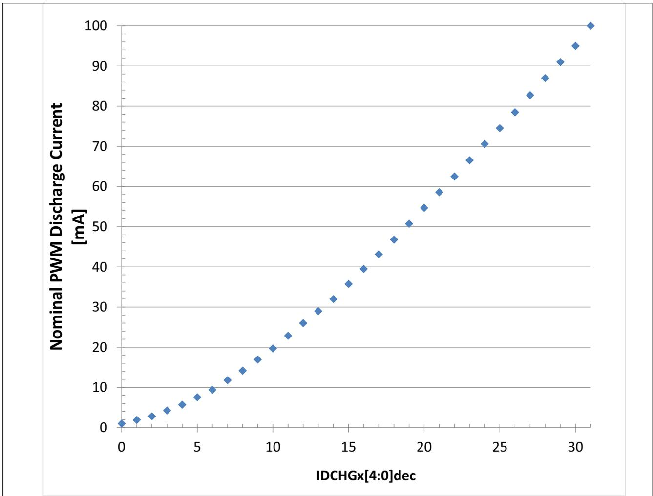
Figure 32 Configurable discharge currents in PWM operation
