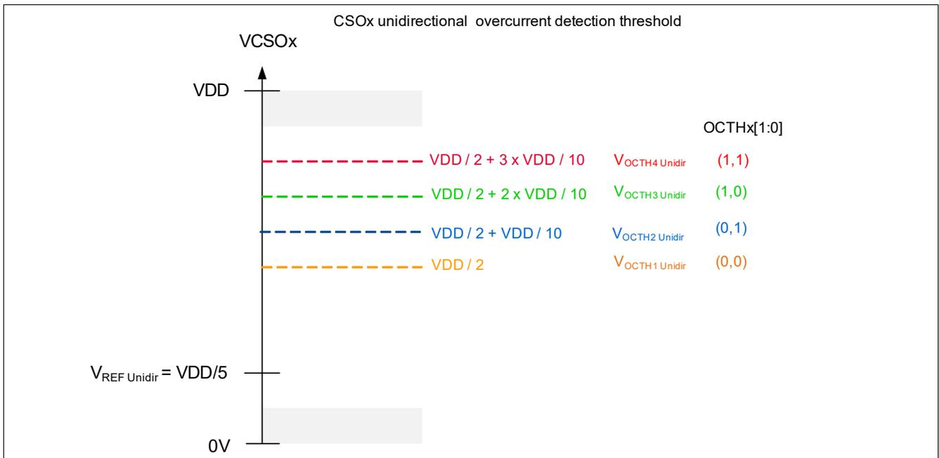
Figure 39 Overcurrent detection thresholds in unidirectional operation (CSDx = 0)
