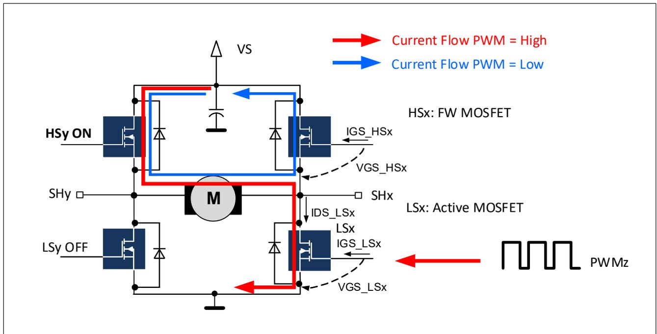
**Figure 19 PWM Channel  $z$  is mapped to low-side  $x$ , motor operating as load**
