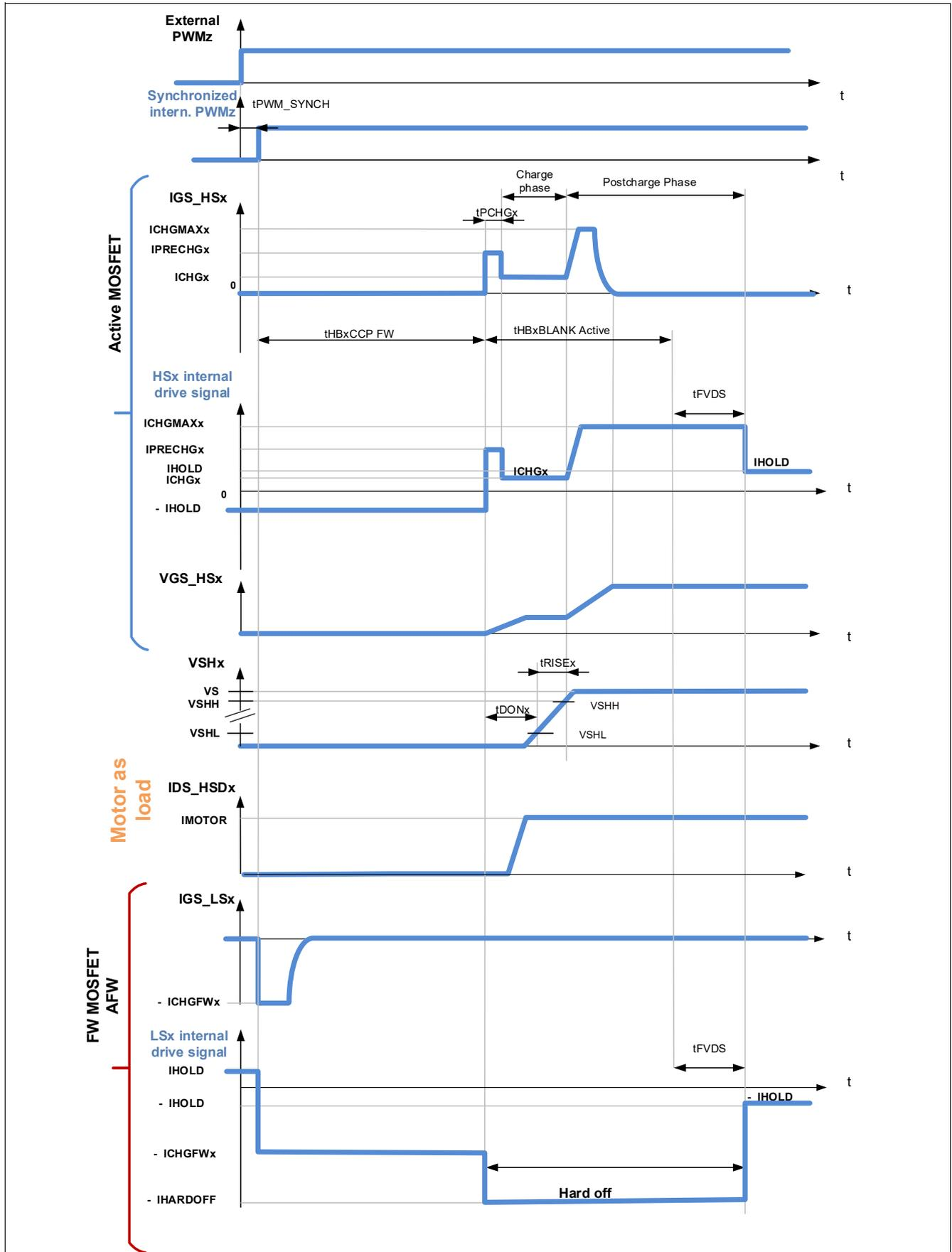
Figure 17 Adaptive turn-on, high-side PWM, AGC[1:0] = (1,0) or (1,1), motor operating as load
