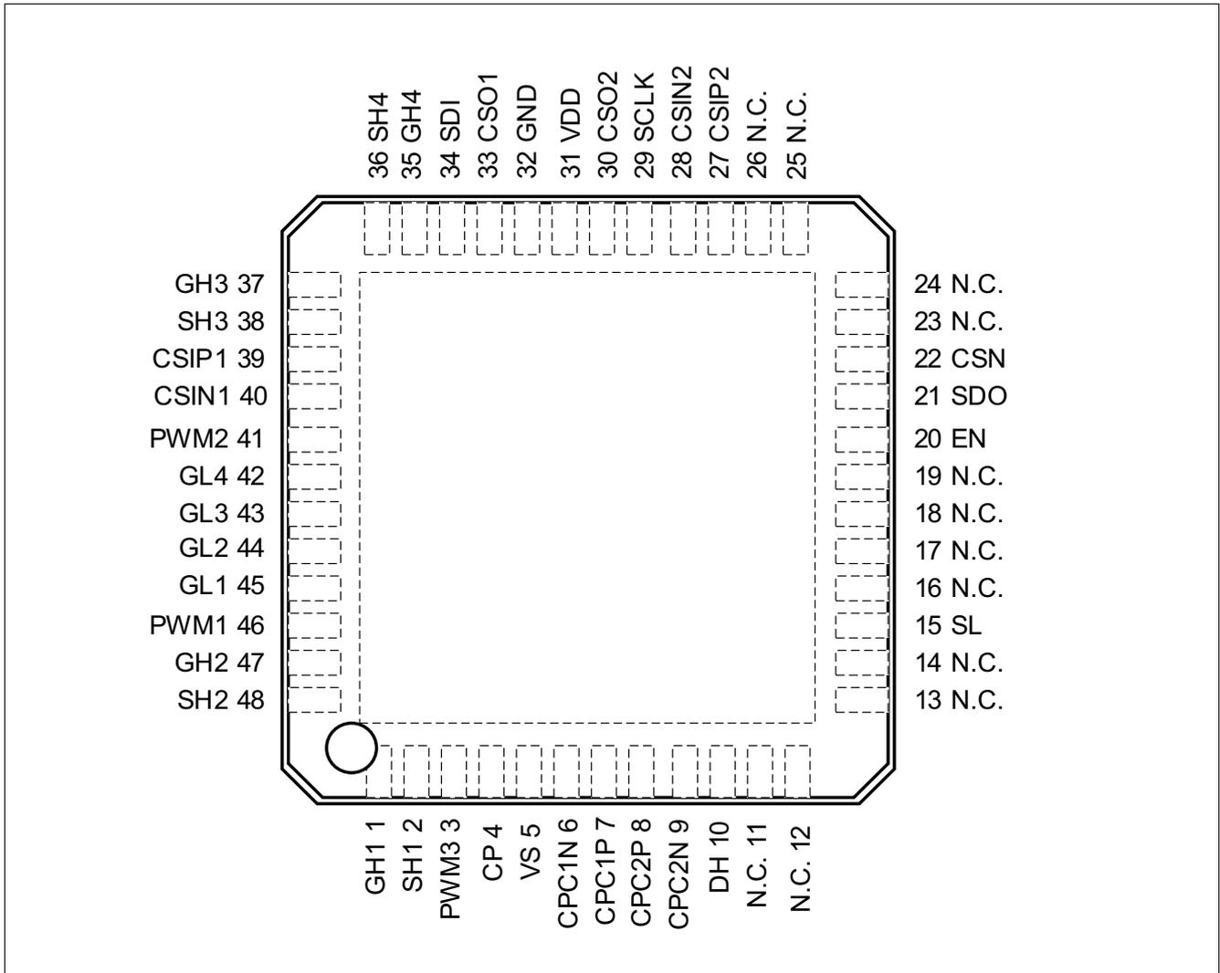
Figure 3 Pin configuration TLE92104-232QX
