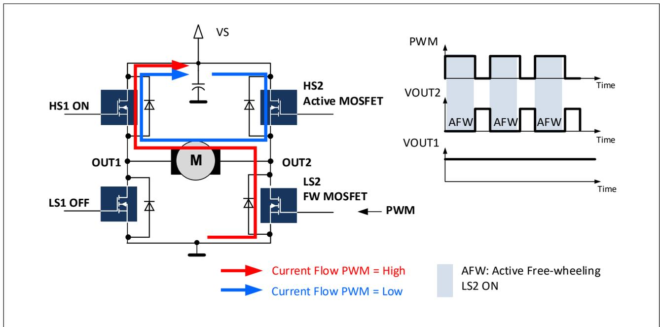
Figure 14 Active freewheeling on HB2: PWM1EN = 1. PWM applied to LS2 (HB2MODE[1:0] = 01<sub>B</sub>). The motor operates as generator: HS2 is the active MOSFET, LS2 is the FW MOSFET.
