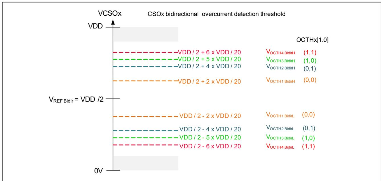
**Figure 40** Overcurrent detection thresholds in bidirectional operation (CSDx = 1)
