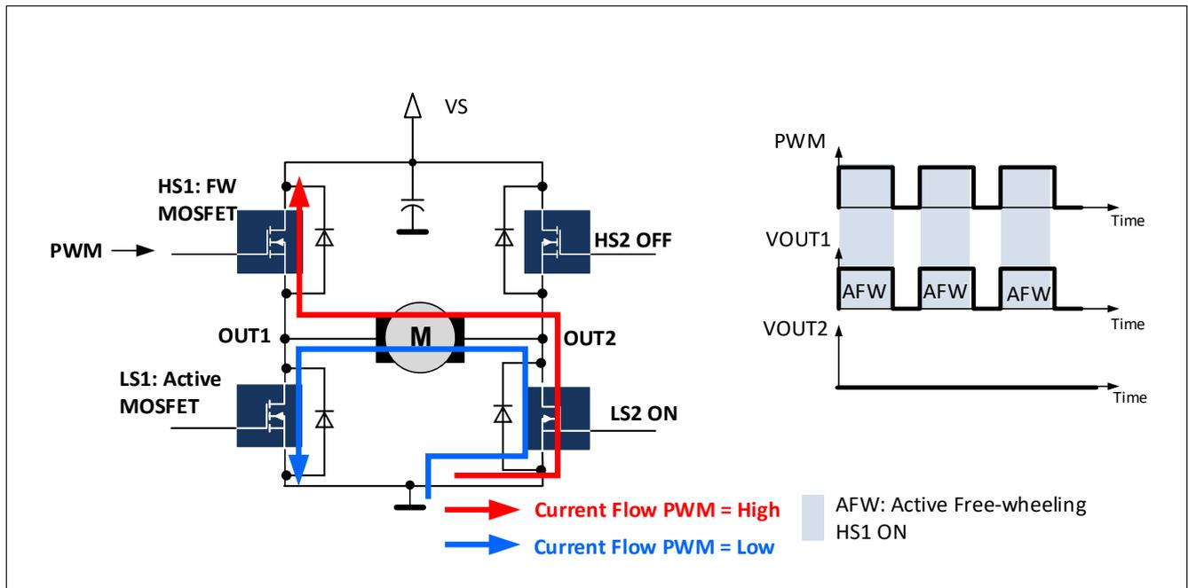
Figure 13 Active freewheeling on HB1: PWM1EN = 1. PWM applied to HS1 (HB1MODE[1:0] = 10<sub>B</sub>). The motor operates as generator: LS1 is the active MOSFET, HS1 is the FW MOSFET.
