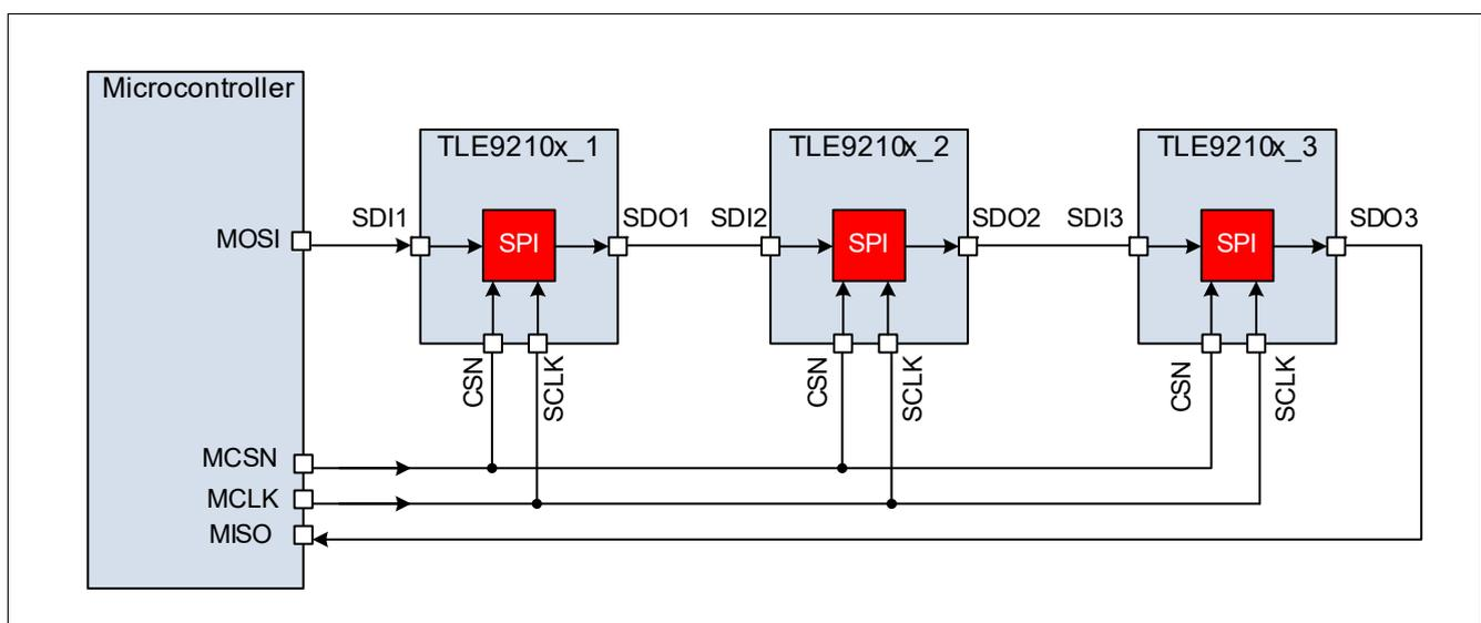
**Figure 46** Daisy chain configuration with three TLE9210x devices
