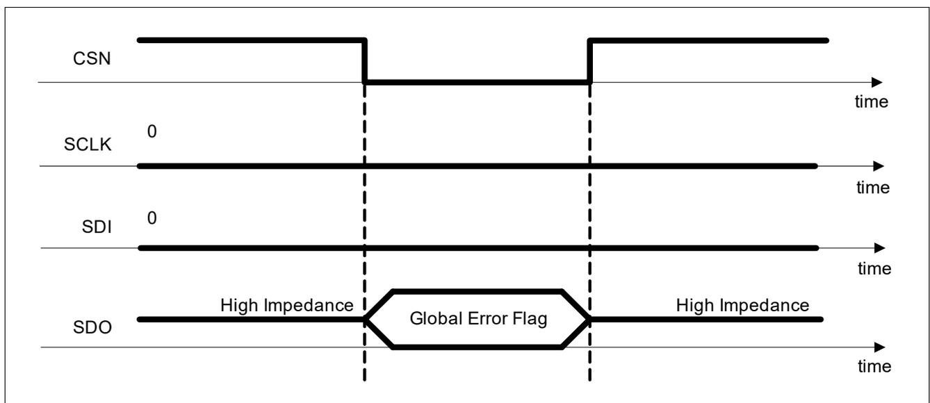
Figure 44 GEF - Diagnostic with 0-clock cycle
