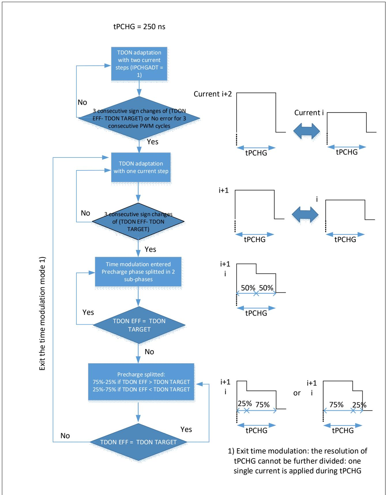
Figure 25 Criteria to exit the time modulation,  $EN\_DEEP\_AD = 1$
