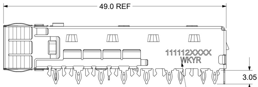
PART NO. AND WEEK/YEAR DATE CODE TO BE PRINTED ON COMPLETED CAGE ASSEMBLY APPROXIMATELY AS SHOWN. SEE TABLE FOR DATE CODE INFORMATION.
