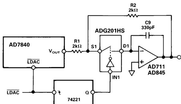
Figure 12. Sample-and-Hold Circuit
