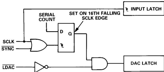
Figure 9. AD7840 Simplified Serial Input Control Logic
