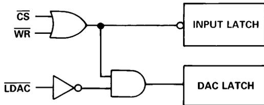
Figure 7. AD7840 Simplified Parallel Input Control Logic
