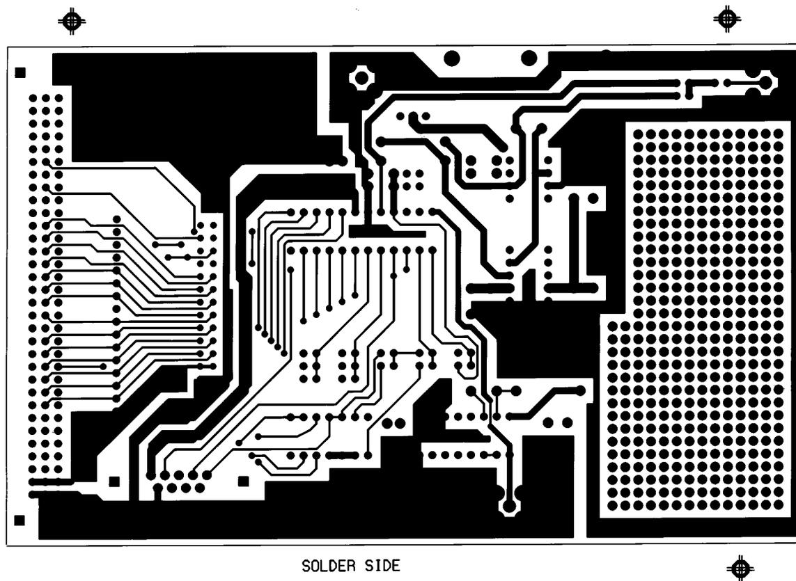
Figure 28. PCB Solder Side Layout for Figure 25
