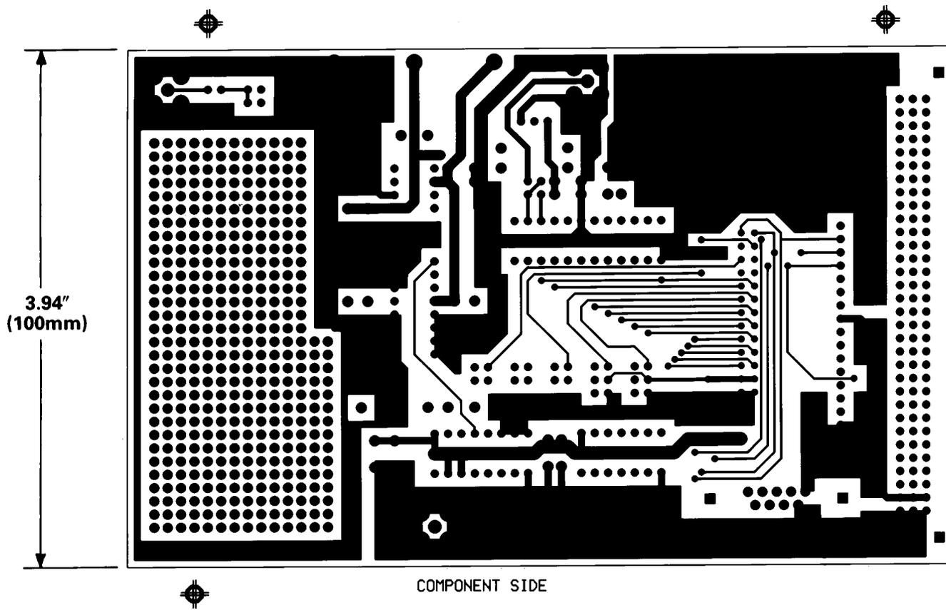
Figure 27. PCB Component Side Layout for Figure 25
