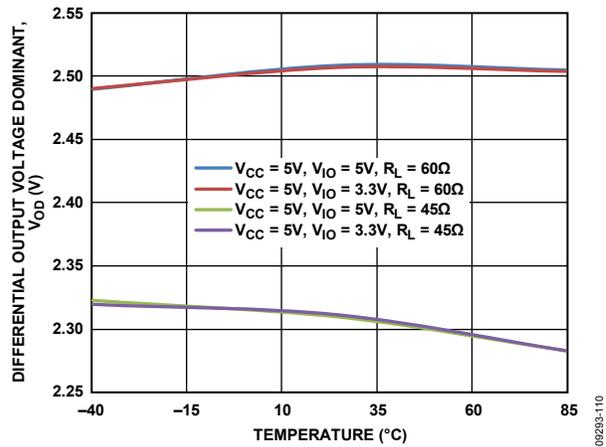
Figure 15. Differential Output Voltage Dominant vs. Temperature
