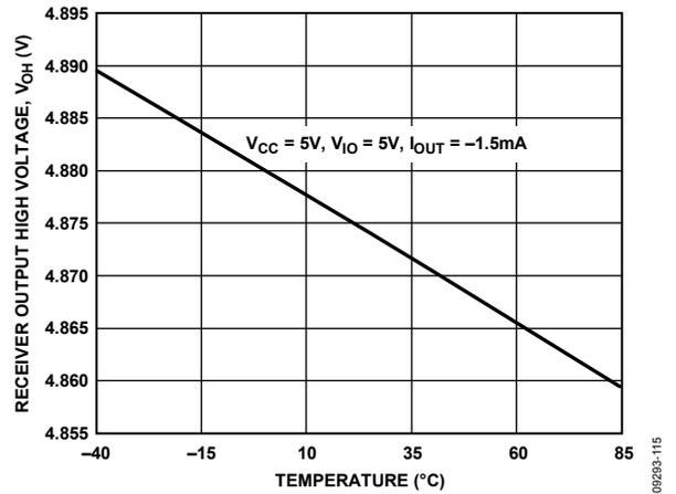
Figure 20. Receiver Output High Voltage vs. Temperature
