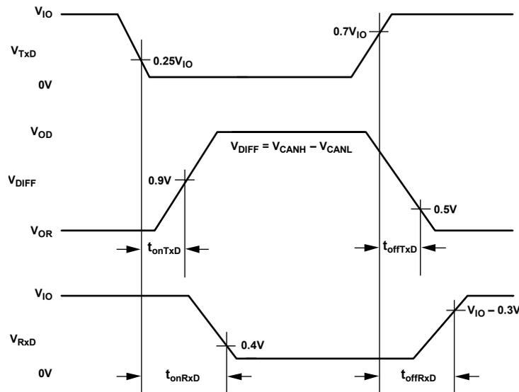
Figure 2. Driver Propagation Delay, Rise/Fall Timing
