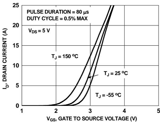
Figure 5. Transfer Characteristics
