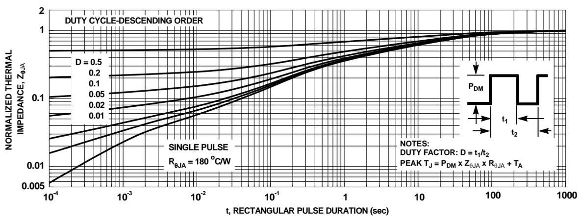
**Figure 11. Junction-to-Ambient Transient Thermal Response Curve**
