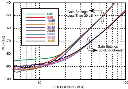
**Figure 10. IM3 vs. Frequency & Gain, High Linearity Bias Setting [6][7]**
