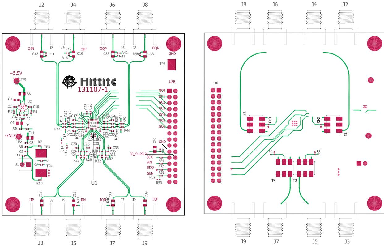
The circuit board used in the application should use RF circuit design techniques. Signal lines should have 50 Ohms impedance while the package ground leads and exposed paddle should be connected directly to the ground plane similar to that shown. A sufficient number of via holes should be used to connect the top and bottom ground planes. The evaluation circuit board shown is available from Hittite upon request.
