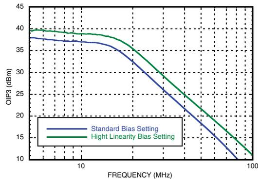
**Figure 14. Output IP3 vs. Frequency & Bias, Gain = 30 dB [5][6] [7] [9]**
