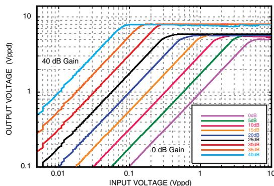
**Figure 18. Output vs. Expected Output Over Gain [8]**
