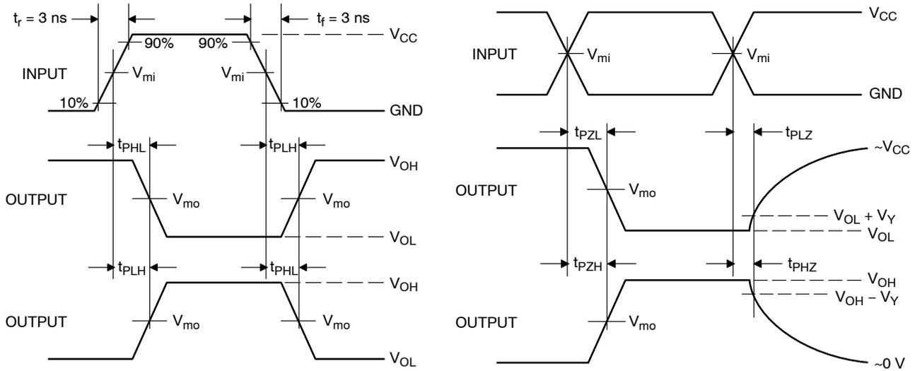
**Figure 4. Switching Waveforms**
