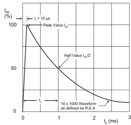
Fig. 4. Pulse waveform
