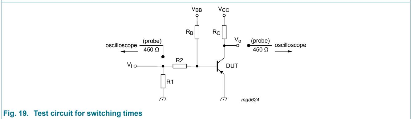
Fig. 19. Test circuit for switching times
