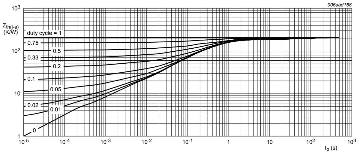
4-layer PCB 35  $\mu\text{m}$ , standard footprint
