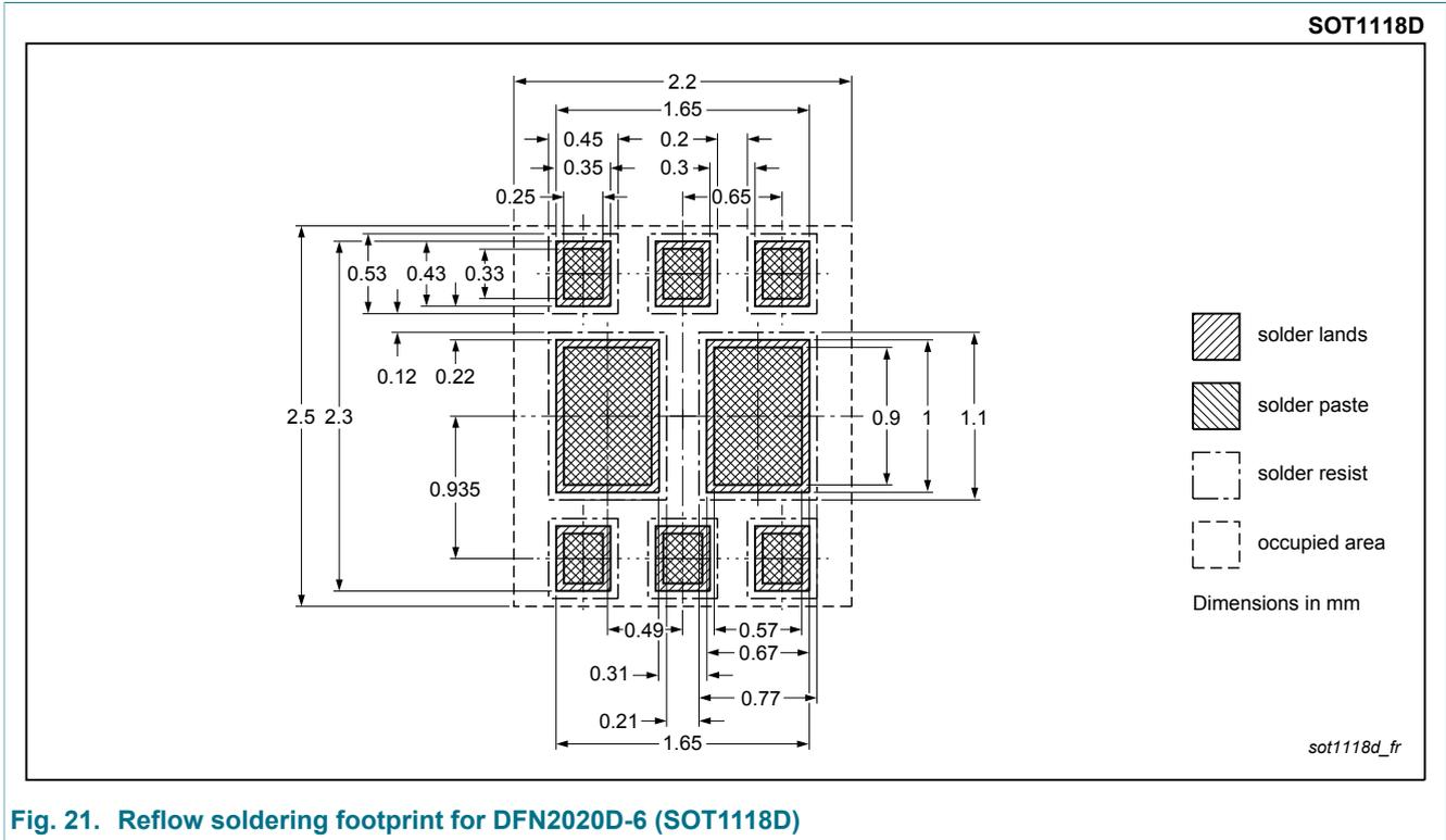
**Fig. 21. Reflow soldering footprint for DFN2020D-6 (SOT1118D)**
