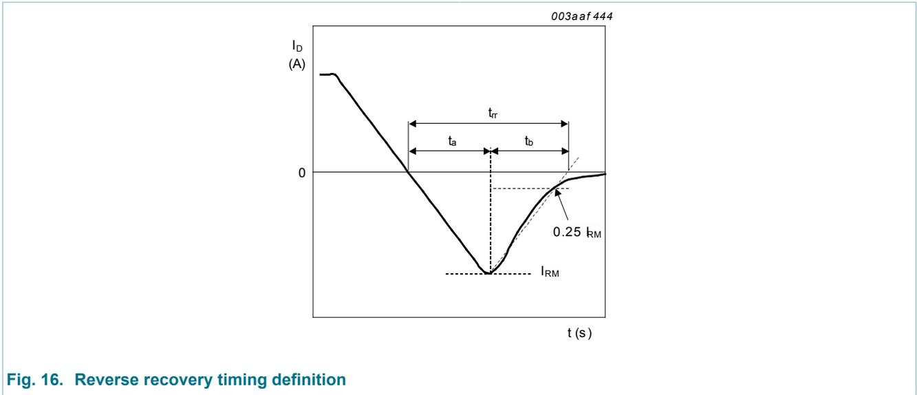
Fig. 16. Reverse recovery timing definition
