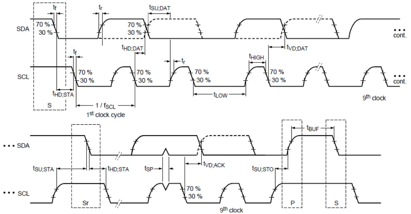
Figure 5.1. I<sup>2</sup>C Serial Port Timing Standard and Fast Modes
