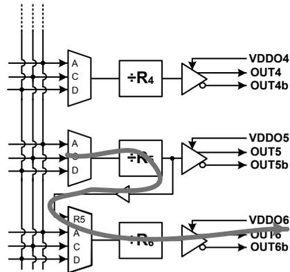
**Figure 3.18. Generating a 1 Hz Output using the Si5348**
