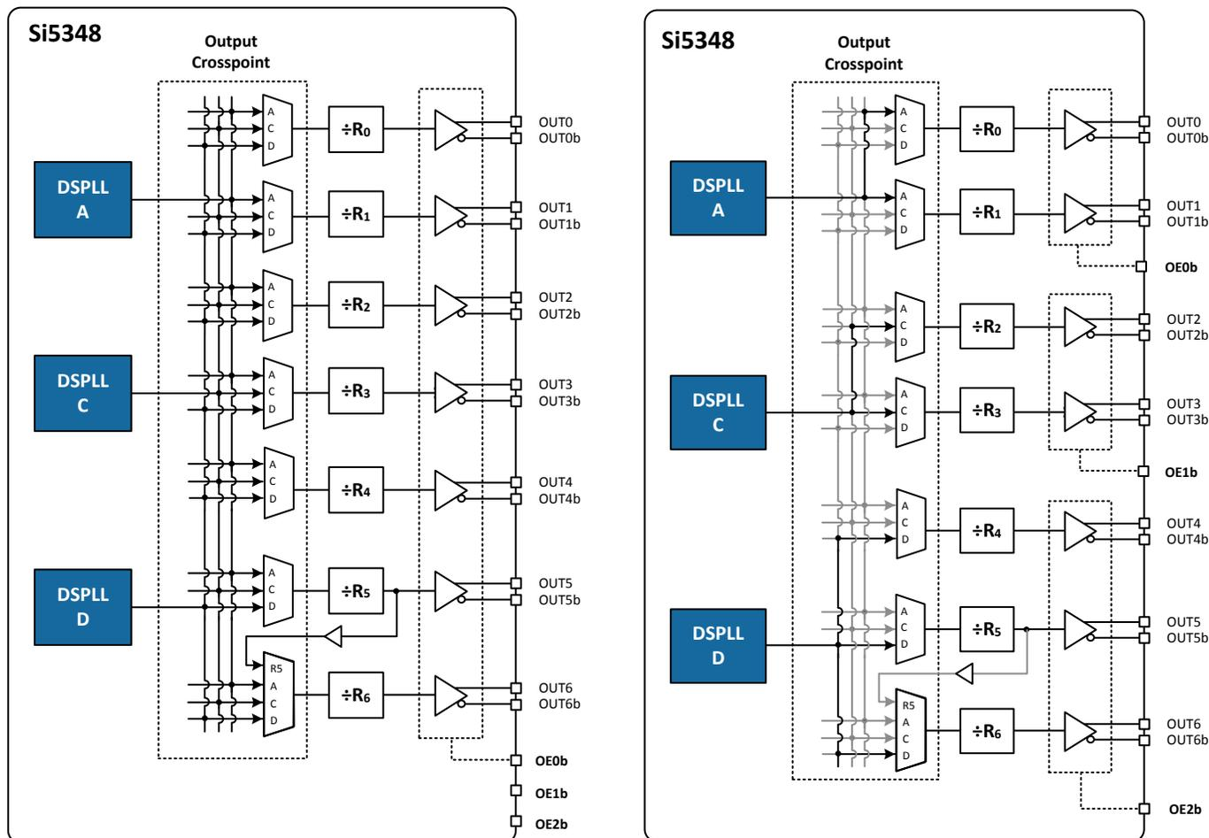
In its default state the OE0b pin enables/disables all outputs. The OE1b and OE2b pins are not mapped and have no effect on outputs.
