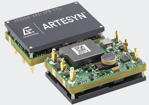
Advanced Energy's Artesyn AVD200-48S12 is a single output DC/DC converter with standard sixteenth-brick outline and pin configuration. It delivers up to 17A output current with 12V output voltage. Above 93.9% ultra-high peak efficiency and excellent thermal performance makes it an ideal choice to supply power in telecom and datacom applications.
