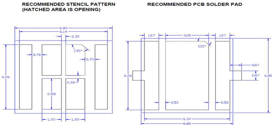
**Figure 1. IN-C68QABTM / IN-C68QACTM Recommended Solder Pattern**
