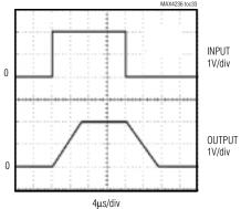
$\begin{aligned} &V_{CC}=\pm 2.5V\\ &R_L=100k\Omega,\ C_L=15pF\\ &A_V=1V/V \end{aligned}$
