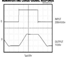
$V_{CC} = \pm 2.5V$   $R_L = 100k\Omega$ ,  $C_L = 15pF$   $A_V = 5V/V$
