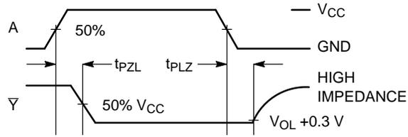
Figure 3. Switching Waveforms
