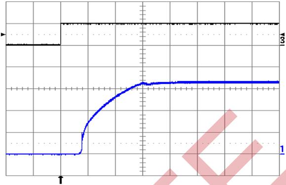
Fig. 8: Turn-on transient at full rated load current (resistive) plus 40,000  $\mu\text{F}$  at  $V_{in} = 48\text{ V}$ , triggered via ON/OFF pin. Top trace: ON/OFF signal (5 V/div.). Bottom trace: output voltage (1 V/div.). Time scale: 2 ms/div.
