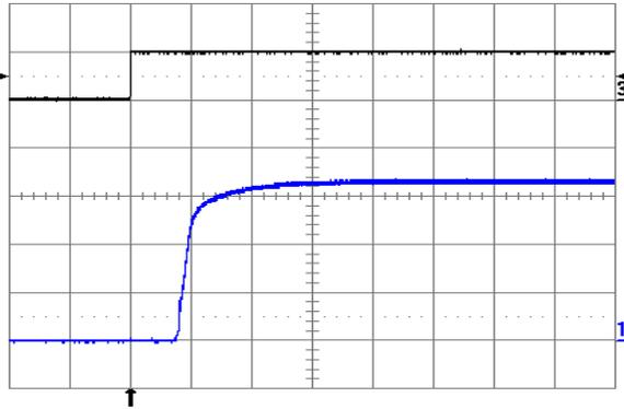
Fig. 7: Turn-on transient at full rated load current (resistive) with no output capacitor at  $V_{in} = 48\text{ V}$ , triggered via ON/OFF pin. Top trace: ON/OFF signal (5 V/div.). Bottom trace: output voltage (1 V/div.) Time scale: 2 ms/div.
