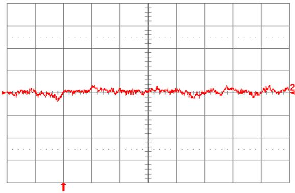
Fig. 12: Input reflected ripple current,  $i_s$  (10 mA/div), measured through 10  $\mu$ H at the source at full rated load current and  $V_{in} = 48$  V. Refer to Fig. 11 for test setup. Time scale: 1  $\mu$ s/div.
