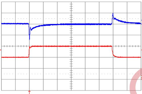
Fig. 9: Output voltage response to load current step-change (20 A – 30 A – 20 A) at  $V_{in} = 48\text{ V}$ . Top trace: output voltage (100 mV/div.). Bottom trace: load current (10 A/div.). Current slew rate: 1 A/ $\mu\text{s}$ .  $C_o = 470\ \mu\text{F}$  tantalum + 1  $\mu\text{F}$  ceramic. Time scale: 0.2 ms/div.
