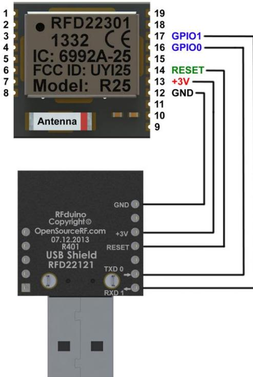
Here is the wiring diagram for the RFD22301 RFduino SMT Module for connecting to the RFD22121 USB programming (shield) dongle.
