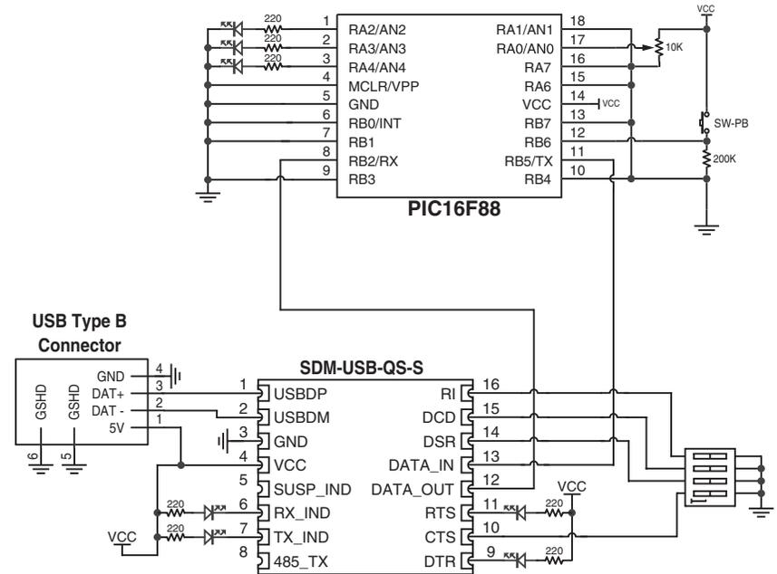
Figure 14: Interface with a Microprocessor
