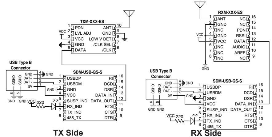
Figure 13: Wireless Modem Using ES Series RF Modules
