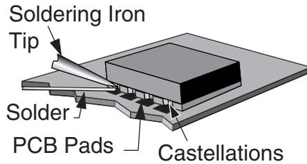
Figure 15: Soldering Technique
