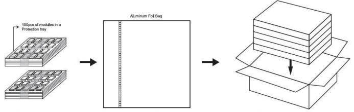
Pack 2 Protection trays (200pcs of modules) into an Aluminum Foil Bag. Seal the Aluminum Foil Bag.
