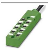
Sensor/actuator box, application: Standard, connection method: M8 socket Metal, number of slots: 8, number of positions: 4, coding: A - standard, slot assignment: Double, status display: yes, pnp; master cable connection: Fixed connection 180°, PUR/PVC, cable length: 5 m, shielding: no
