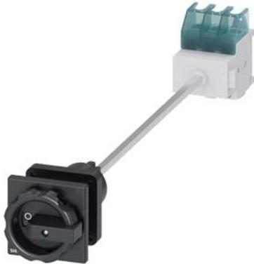
SETRON, Switch disconnecter 3LD, main switch, 3-pole, Iu: 25 A, Operating power / at AC-23 A at 400 V: 9.5 kW, floor mounting with door coupling, rotary operating mechanism, black, central mounting 22.5 mm of the handle
