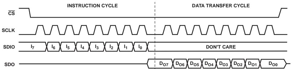
Figure 61. 3-Wire Serial Port Read Timing—Clock Stall Low
