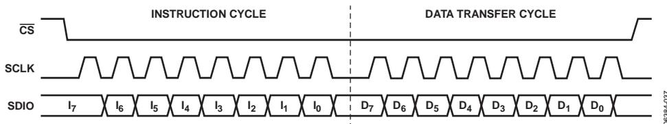
Figure 60. Serial Port Write Timing—Clock Stall Low
