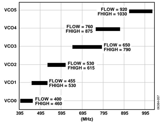
Figure 50. VCO Ranges Including Atypical Wafer Process Skew
