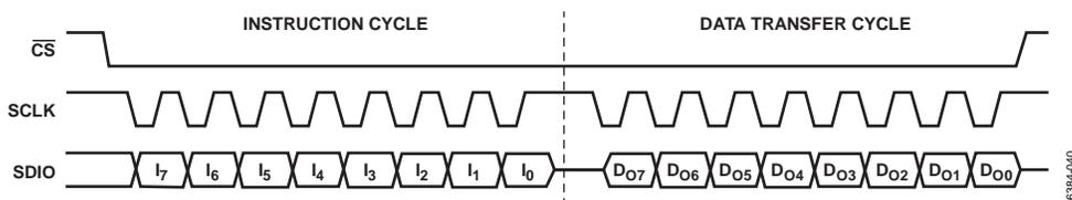
Figure 63. 2-Wire Serial Port Read Timing—Clock Stall High
