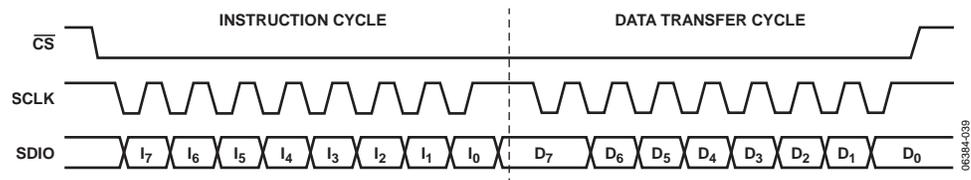
Figure 62. Serial Port Write Timing—Clock Stall High
