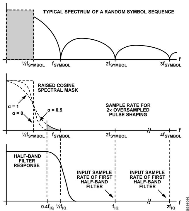
Figure 36. Effect of the Excess Bandwidth Factor ( $\alpha$ )
