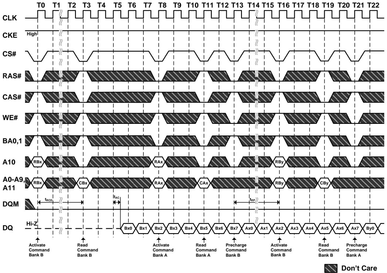
**Figure 30. Random Row Write (Interleaving Banks)**
