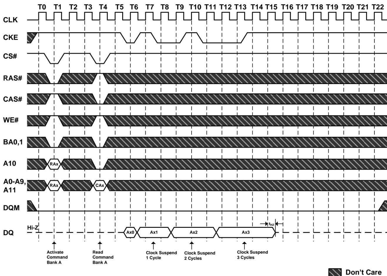
**Figure 25. Clock Suspension During Burst Write (Using CKE)**
