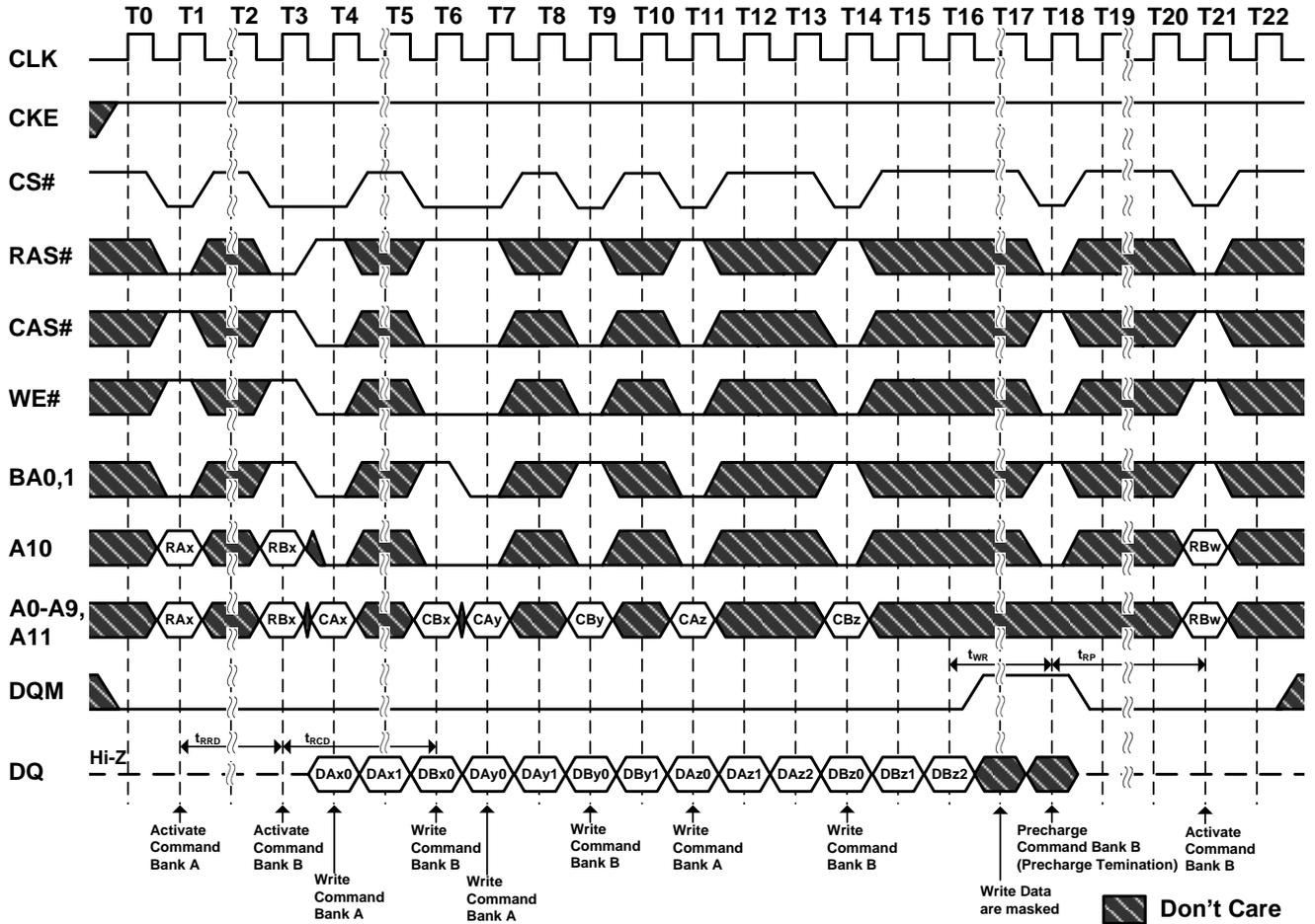
**Figure 42 Precharge Termination of a Burst**
