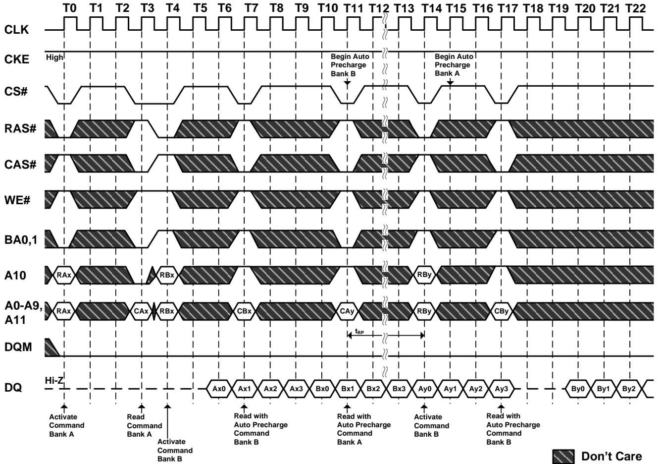
**Figure 35. Auto Precharge after Write Burst (Burst Length=4)**
