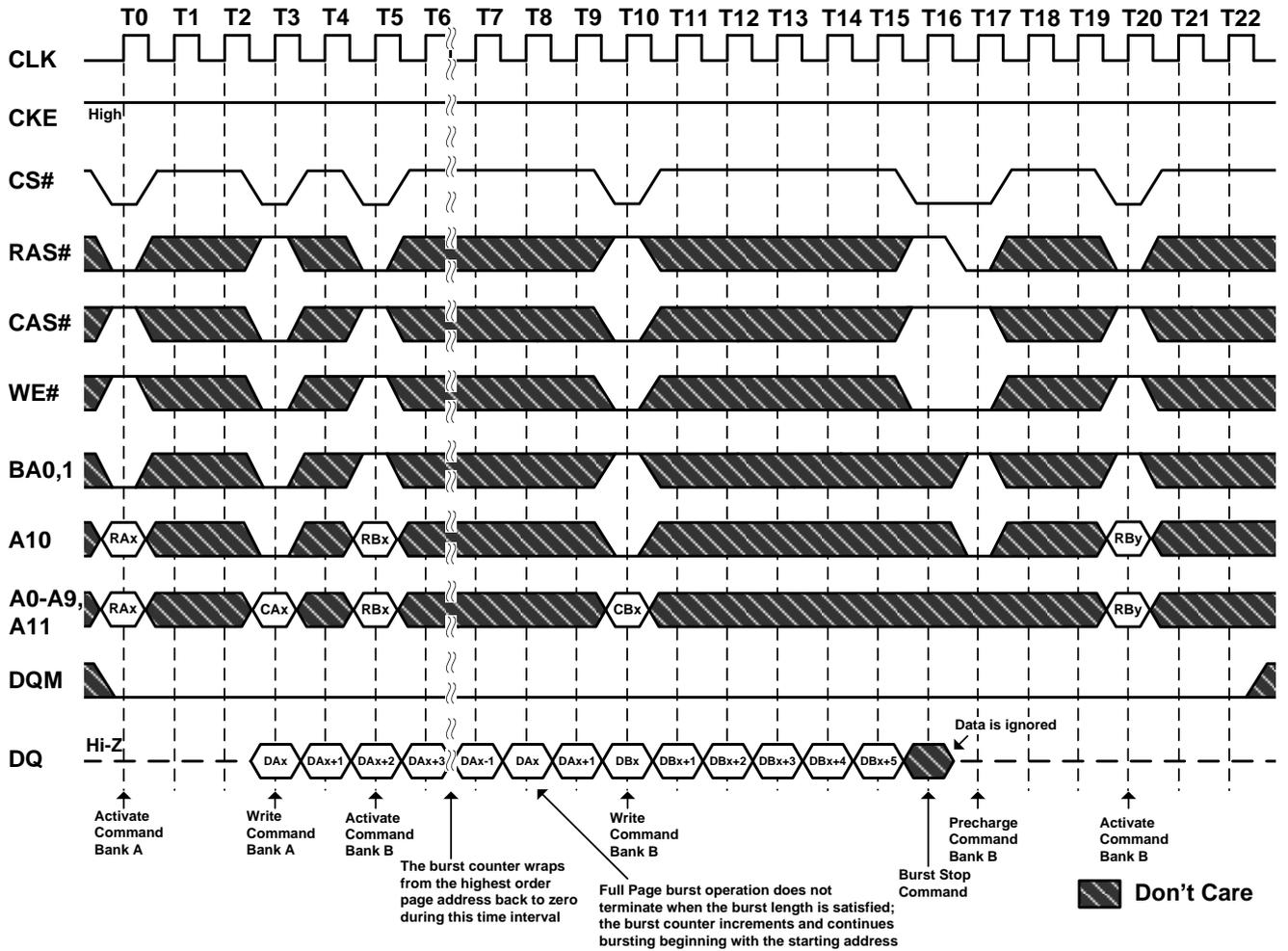
**Figure 38. Byte Read and Write Operation (Burst Length=4, CAS# Latency=2)**
