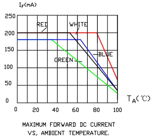
The graph shows the maximum allowable DC current for a LED die of each color.
