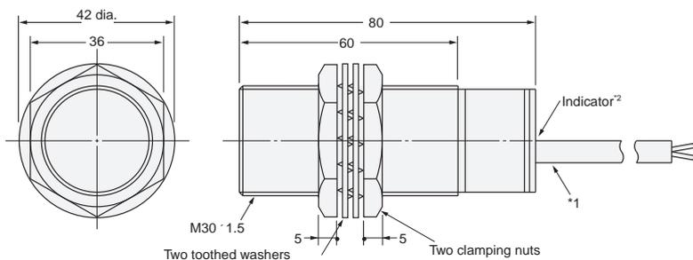
\*1. 6-dia. vinyl-insulated round cable with 3 conductors (Conductor cross section: 0.5 mm<sup>2</sup>, Insulator diameter: 1.9 mm), Standard length: 2 m
