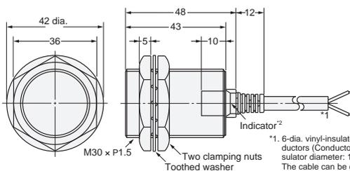
\*1. 6-dia. vinyl-insulated round cable with 2 conductors (Conductor cross section: 0.5 mm<sup>2</sup>, Insulator diameter: 1.9 mm), Standard length: 2 m
