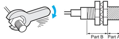
Note: 1. The allowable tightening strength depends on the distance from the edge of the head, as shown in the following table. (A is the distance from the edge of the head. B includes the nut on the head side. If the edge of the nut is in part A, the tightening torque for part A applies instead.)
