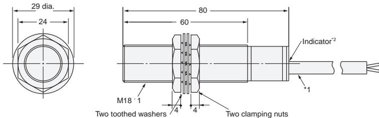
\*1. 6-dia. vinyl-insulated round cable with 3 conductors (Conductor cross section: 0.5 mm<sup>2</sup>, Insulator diameter: 1.9 mm), Standard length: 2 m
