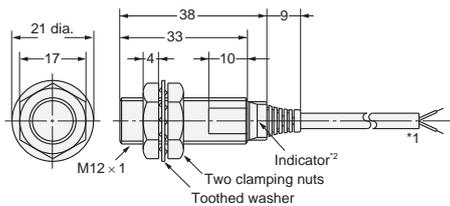
\*1. 4-dia. vinyl-insulated round cable with 2 conductors (Conductor cross section: 0.3 mm<sup>2</sup>, Insulator diameter: 1.3 mm), Standard length: 2 m
