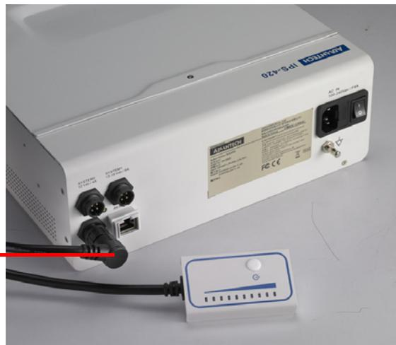
**Figure 2.7 Connecting the remote control**
