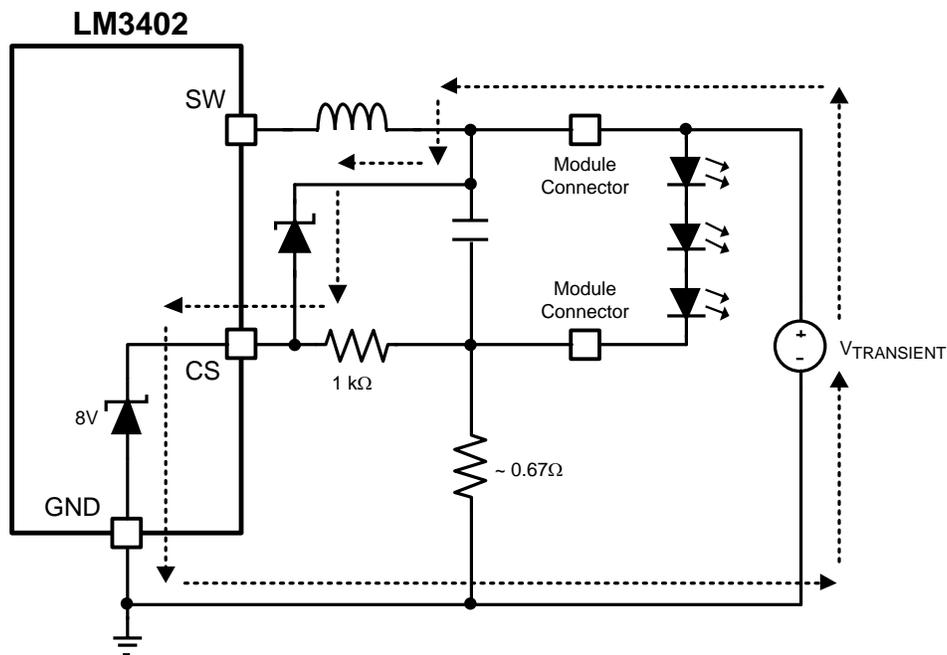
Figure 24. CS Pin With OVP, Transient Path
