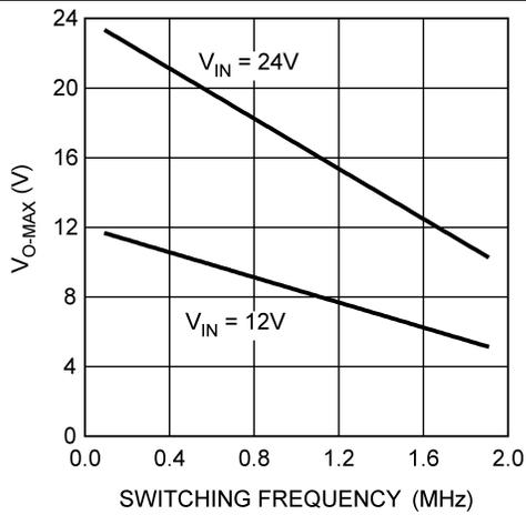
Figure 13. V<sub>O-MAX</sub> vs f<sub>SW</sub>, LM3402 (T<sub>A</sub> = 25°C)
