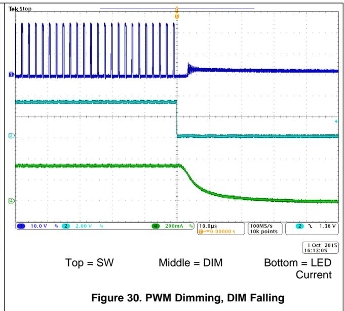
**Figure 30. PWM Dimming, DIM Falling**
