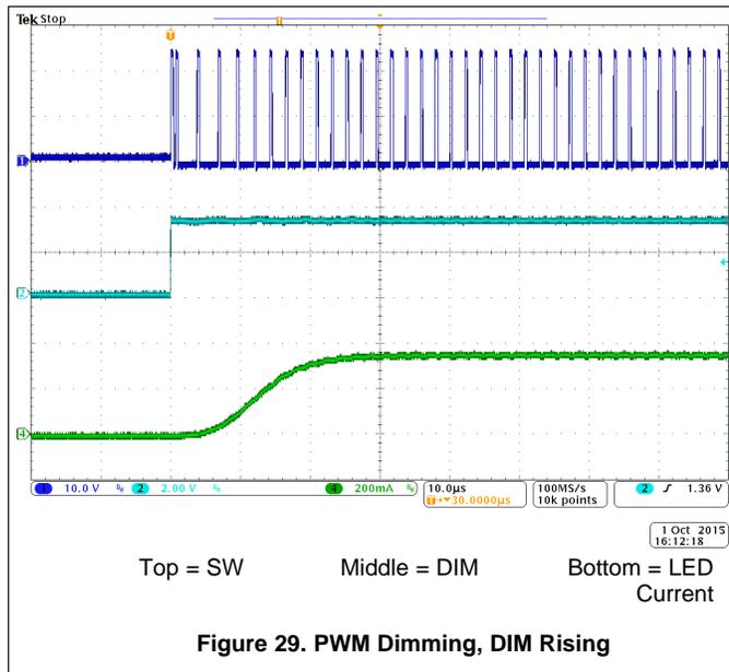
**Figure 29. PWM Dimming, DIM Rising**
