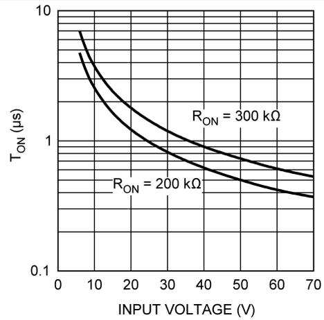
Figure 8.  $T_{ON}$  vs  $V_{IN}$  ( $T_A = 25^\circ\text{C}$ )
