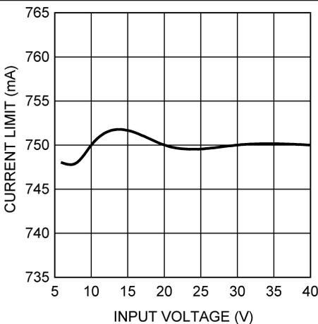
Figure 5. Current Limit vs  $V_{IN}$ , LM3402 ( $T_A = 25^\circ\text{C}$ )
