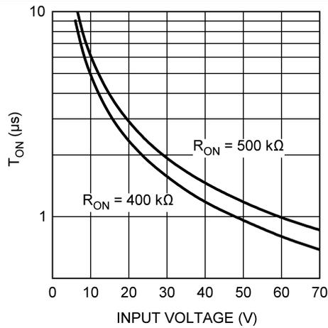
Figure 9.  $T_{ON}$  vs  $V_{IN}$ , ( $T_A = 25^\circ\text{C}$ )
