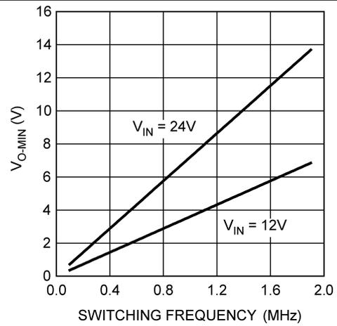
Figure 14. V<sub>O-MIN</sub> vs f<sub>SW</sub>, LM3402 (T<sub>A</sub> = 25°C)
