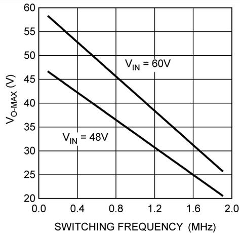
Figure 15. V<sub>O-MAX</sub> vs f<sub>SW</sub>, LM3402HV (T<sub>A</sub> = 25°C)
