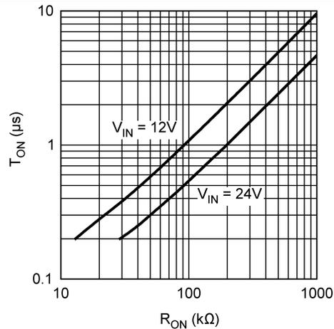
Figure 10.  $T_{ON}$  vs  $R_{ON}$ , LM3402 ( $T_A = 25^\circ\text{C}$ )
