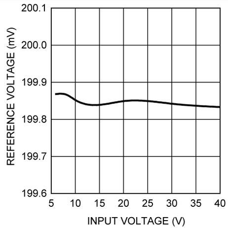
Figure 2.  $V_{REF}$  vs  $V_{IN}$ , LM3402 ( $T_A = 25^\circ\text{C}$ )
