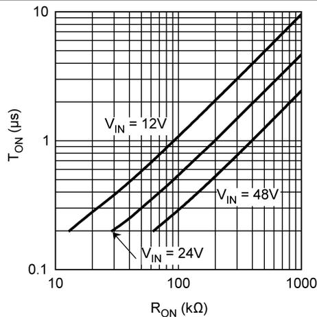
Figure 11.  $T_{ON}$  vs  $R_{ON}$ , LM3402HV ( $T_A = 25^\circ\text{C}$ )
