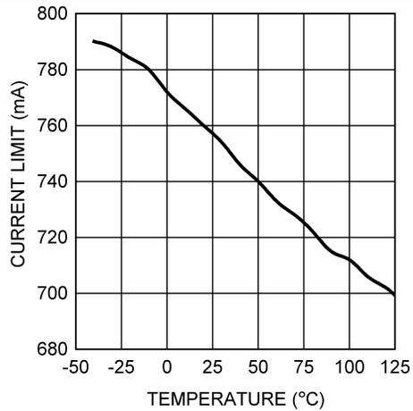
Figure 4. Current Limit vs Temperature ( $V_{IN} = 24$  V)
