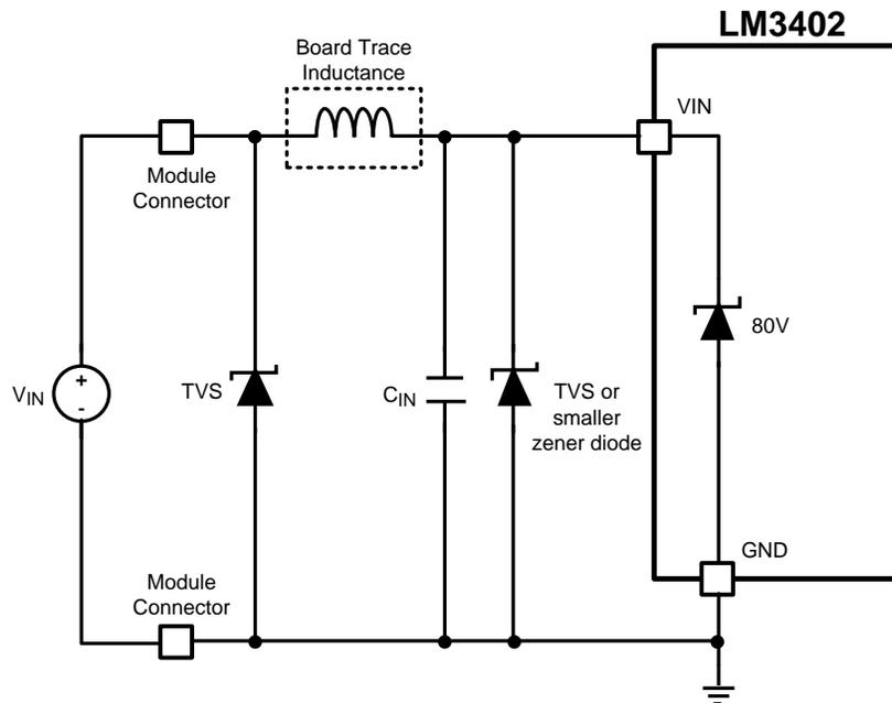
Figure 27. VIN Pin With Additional Input Protection
