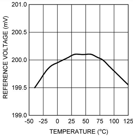
Figure 1.  $V_{REF}$  vs Temperature ( $V_{IN} = 24$  V)
