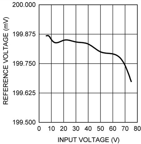
Figure 3.  $V_{REF}$  vs  $V_{IN}$ , LM3402HV ( $T_A = 25^\circ\text{C}$ )
