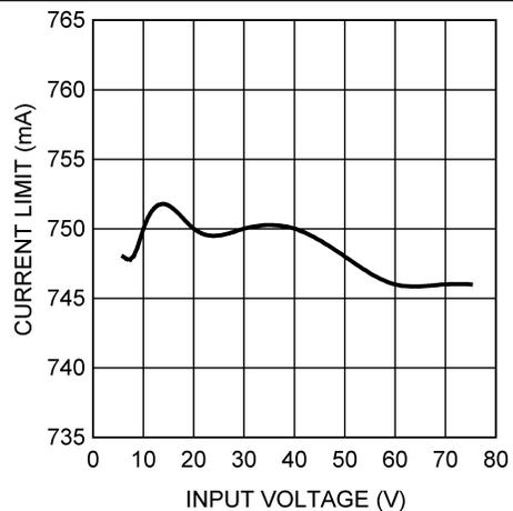
Figure 6. Current Limit vs  $V_{IN}$ , LM3402HV ( $T_A = 25^\circ\text{C}$ )
