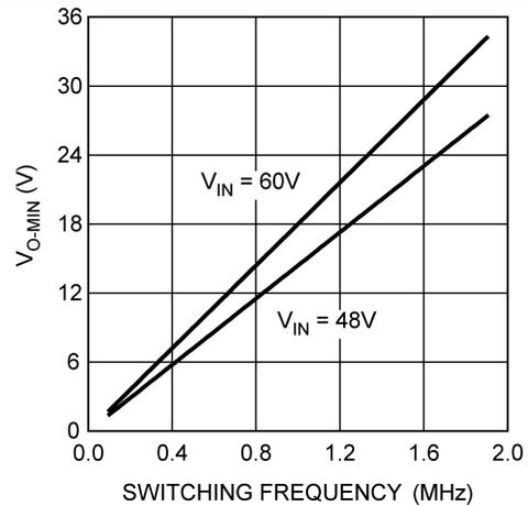
Figure 16. V<sub>O-MIN</sub> vs f<sub>SW</sub>, LM3402HV (T<sub>A</sub> = 25°C)
