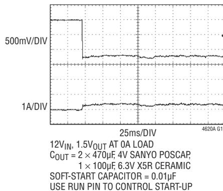
**12V to 1.5V, 13A No Load Short-Circuit Testing**
