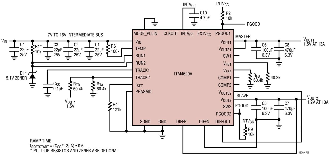
Figure 6. Example of Output Tracking Application Circuit
