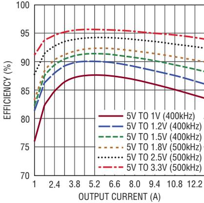
**Efficiency vs Output Current,  $V_{IN} = 8V$**
