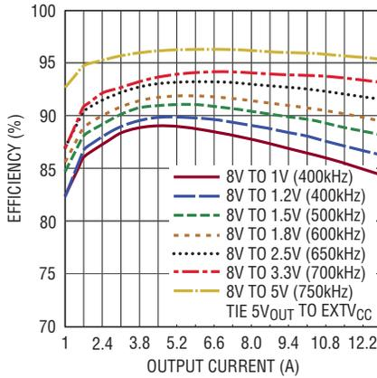
**Efficiency vs Output Current,  $V_{IN} = 12V$**
