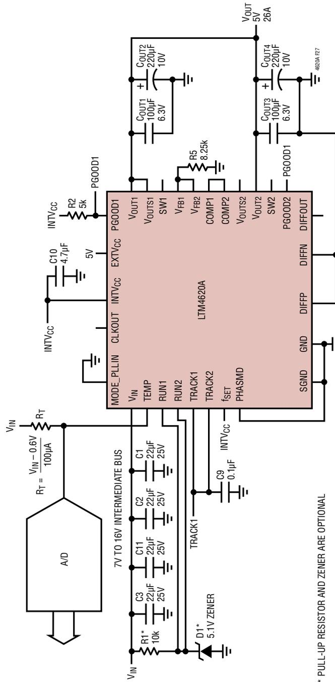
Figure 27. LTM4620A 2-Phase, 5V at 20A Design with Temperature Monitoring
