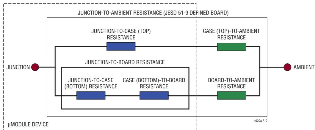
Figure 9. Graphical Representation of JESD 51-12 Thermal Coefficients
