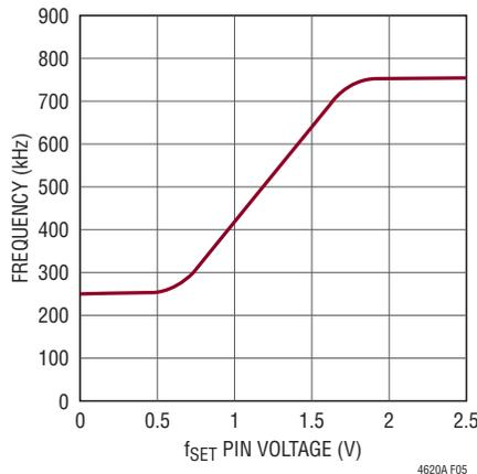
Figure 5. Operating Frequency vs  $f_{SET}$  Pin Voltage
