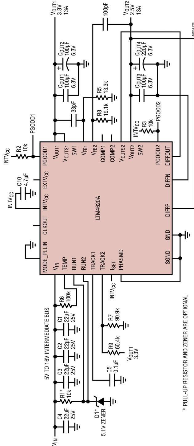
Figure 28. LTM4620A 3.3V and 2.5V Output Tracking
