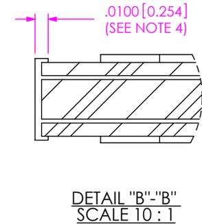
BROKEN EDGE MUST BE LOWER THAN PLATED EDGE OR MILLED FOR HOUSING CLEARANCE.
