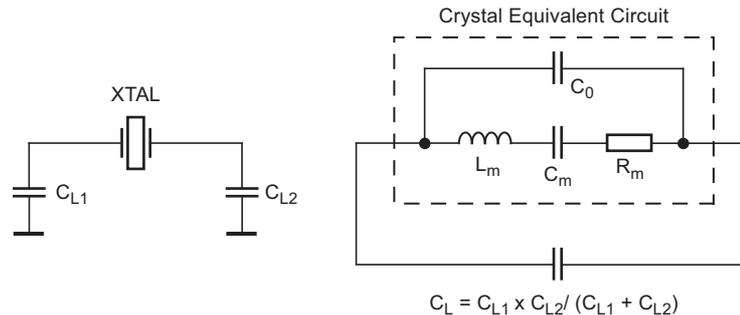
With  $C_m \leq 10\text{fF}$ ,  $C_0 \geq 1.0\text{pF}$ ,  $C_{LN} = 9\text{pF}$  and  $C_{L1,2} = 16\text{pF} \pm 1\%$ , the pulling amounts to  $P \leq \pm 1\text{ppm}$ .
