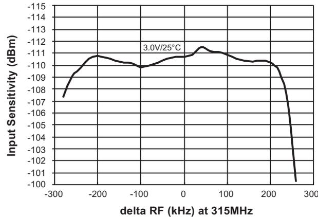
**Figure 2-4. Measured Sensitivity (315MHz, FSK, 2.4Kbits/s, ±38kHz, Manchester) Versus Frequency Offset**
