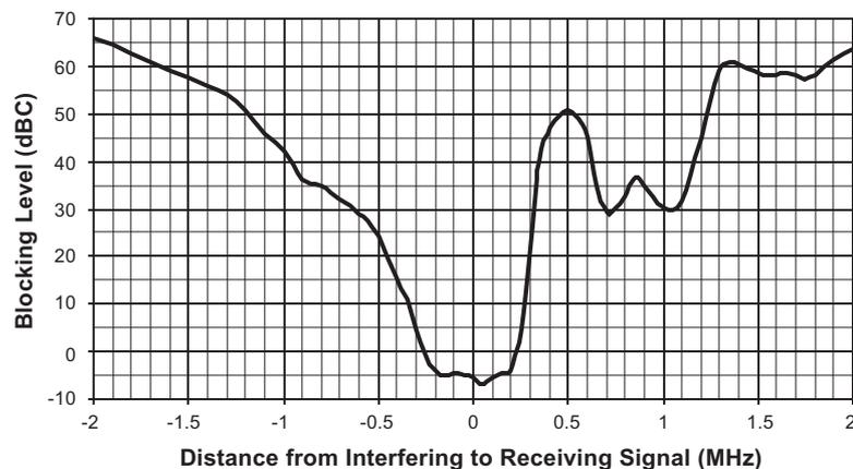
**Figure 2-7. Narrow-band 3-dB Blocking Characteristic at 315MHz**
