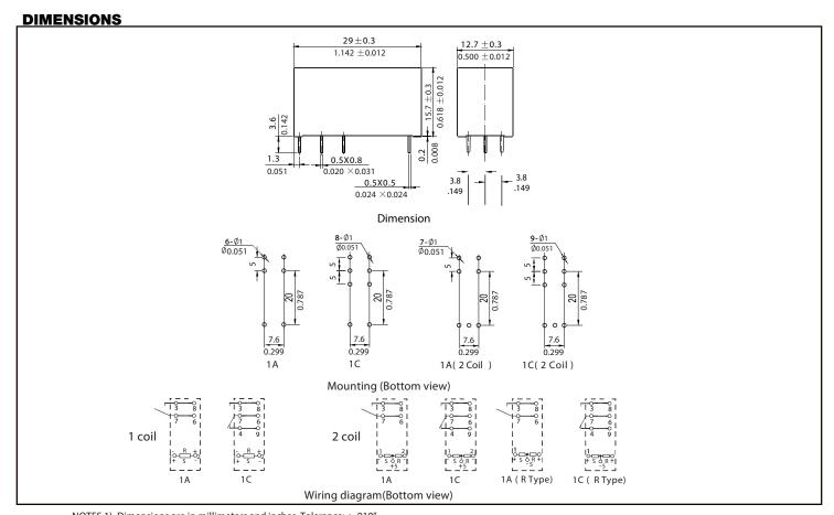
NOTES 1). Dimensions are in millimeters and inches. Tolerance:  $\pm$  .010" 2). Inch equivalents are given for general information only.
