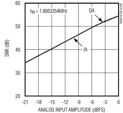
**Rx ADC SIGNAL-TO-NOISE AND DISTORTION RATIO vs. ANALOG INPUT AMPLITUDE**
