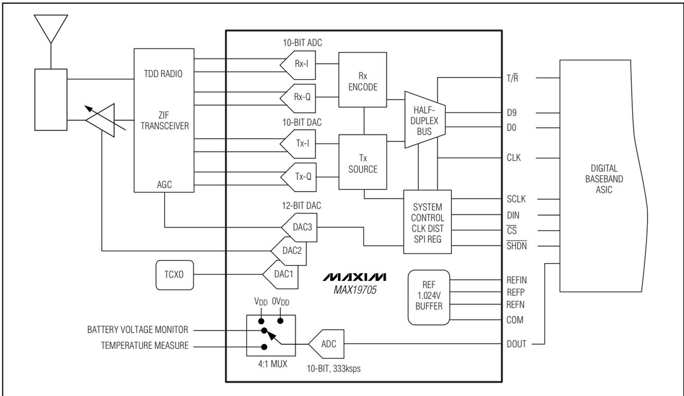
Figure 12. Typical Application Circuit for TDD Radio
