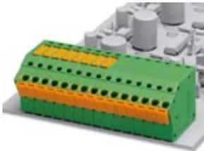
PCB terminal block, Nominal current: 13.5 A, Nom. voltage: 320 V, Pitch: 5.08 mm, Number of positions: 1, Connection method: Spring-cage connection, Mounting: Soldering, Conductor/PCB connection direction: 60 °, Color: green, The article can be aligned to create different nos. of positions!
