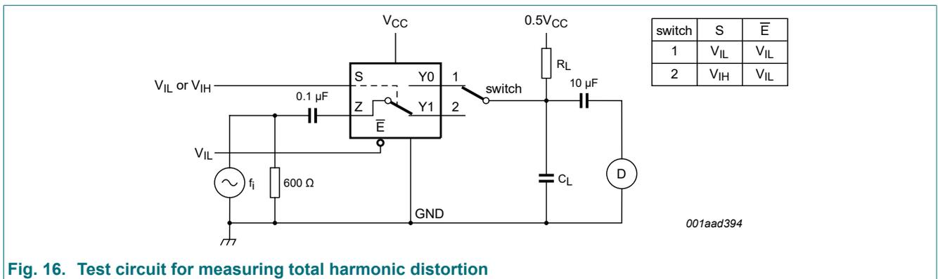
**Fig. 16. Test circuit for measuring total harmonic distortion**
