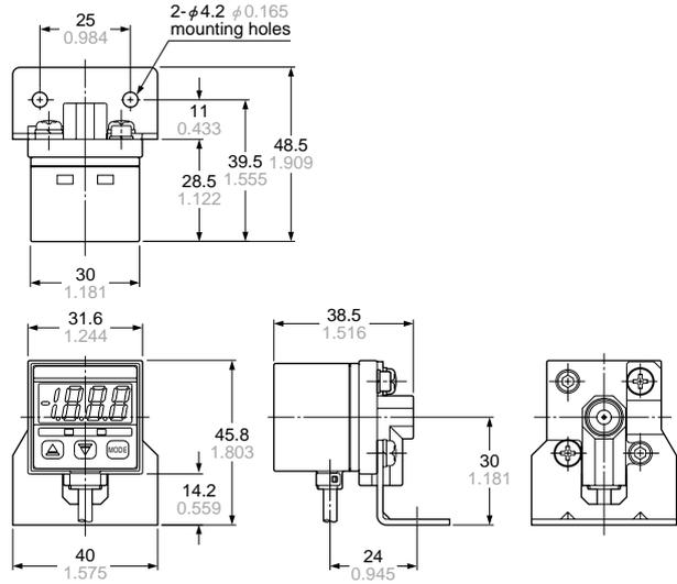
Material: Cold rolled carbon steel (SPCC)
