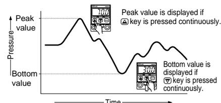
Note: The above graph is for a positive pressure type sensor.
