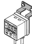
Two M4 (length 6 mm 0.236 in) pan head screws and two spring washers are attached.
