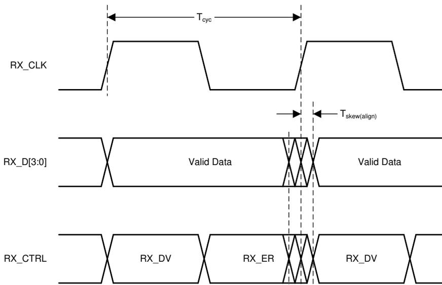
**Figure 6-6. RGMII Receive Timing (Internal Delay Disabled)**
