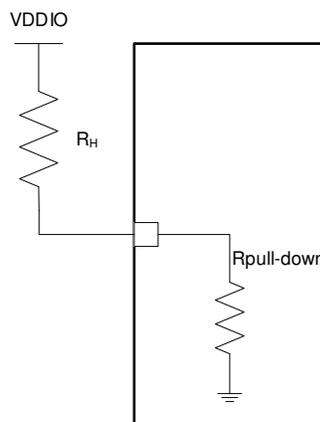
Figure 7-18. Strap Circuit
