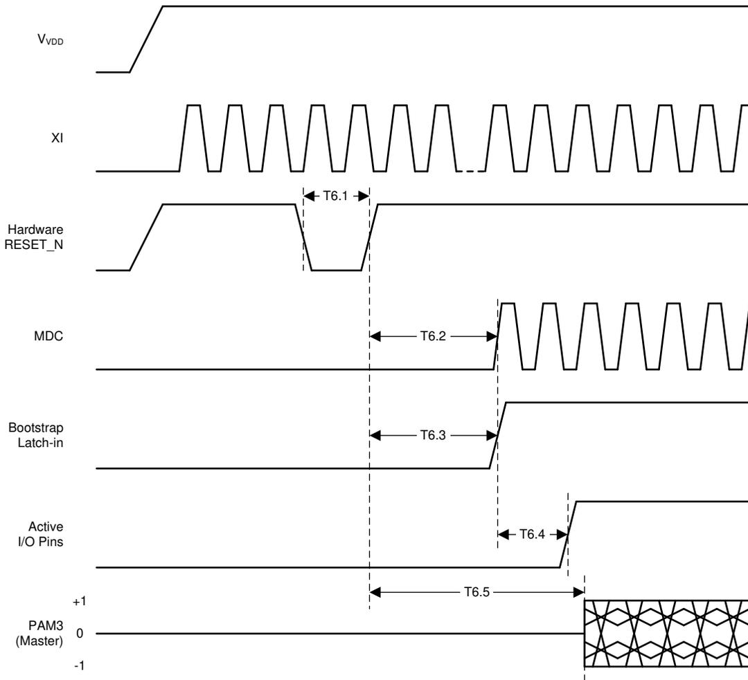
**Figure 6-2. Reset Timing**
