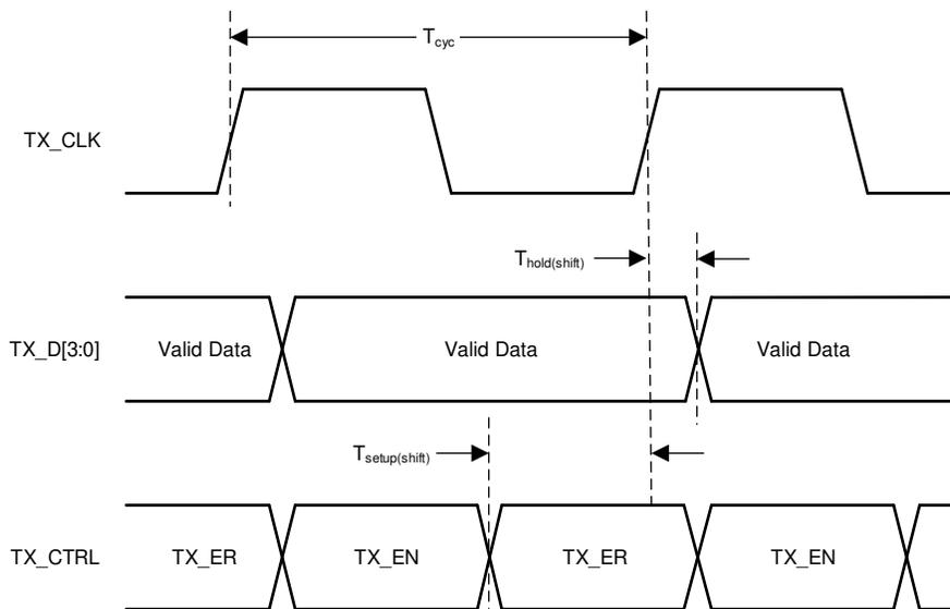
**Figure 6-3. RGMII Transmit Timing (Internal Delay Enabled)**
