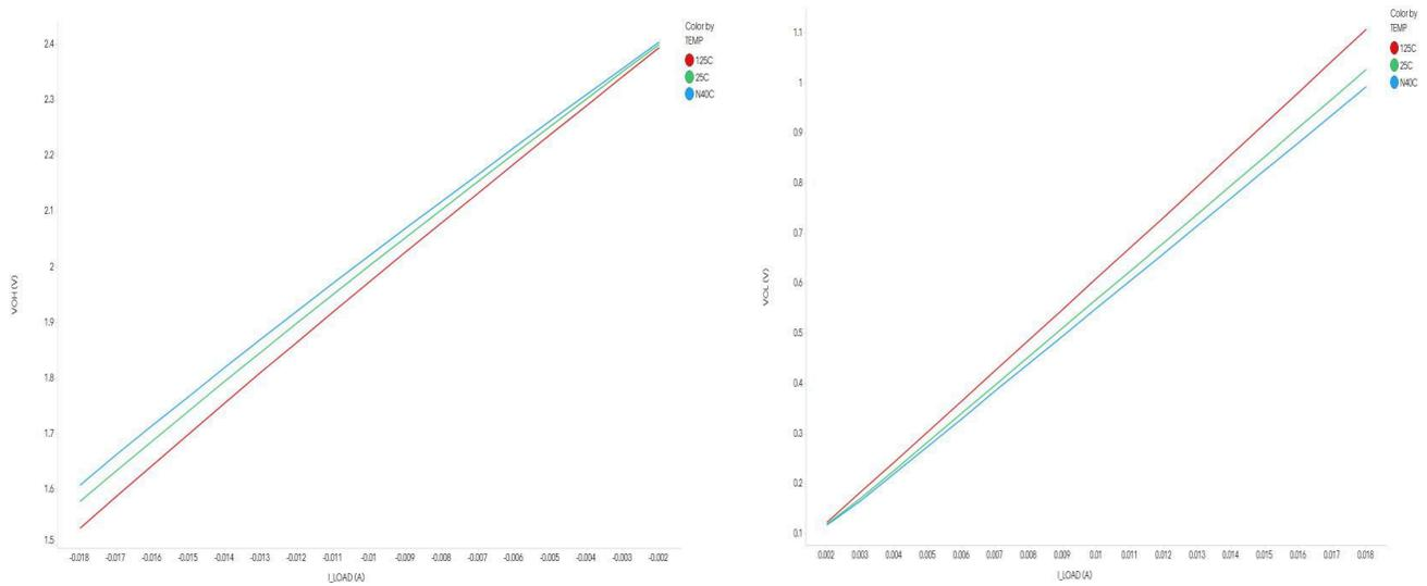
**Figure 6-9. LED V vs I for 2.5V VDDIO**
