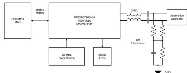
**Figure 3-1. Simplified Schematic**
