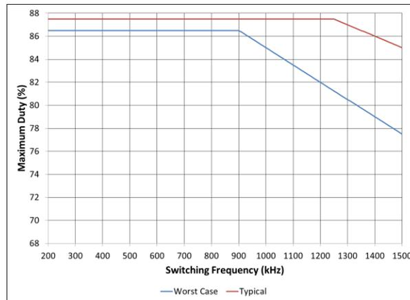
Figure 22: Maximum duty cycle vs. switching frequency
