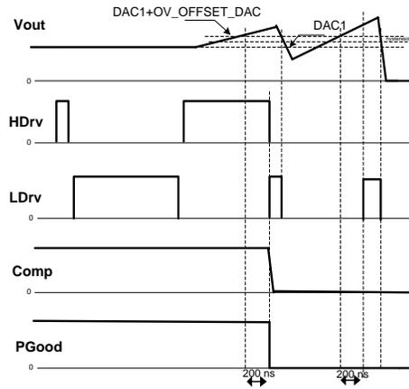
Figure 21: Timing Diagram for OVP in non-tracking mode
