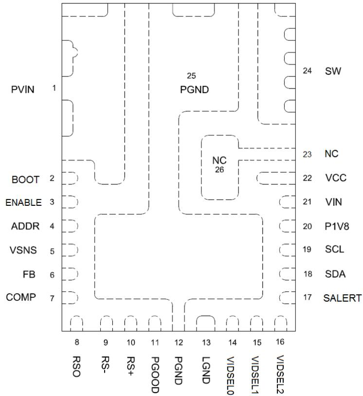
**Figure 2: IR38263 Package Top View
