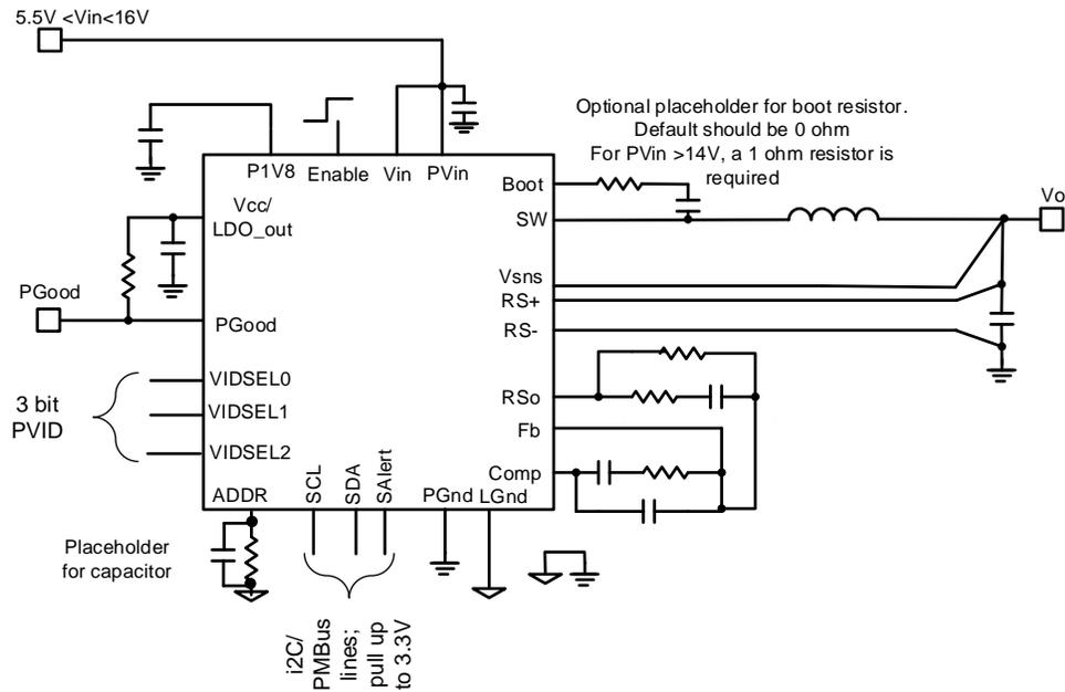
Figure 4: Using the internal LDO,  $V_o < 2.555V$
