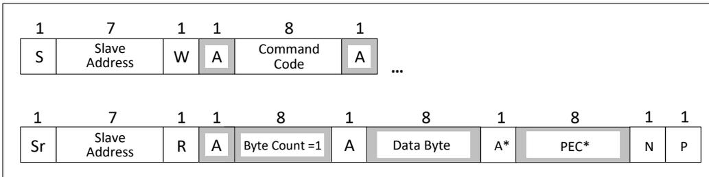
Figure 28: SMBus Block Read with Byte Count=1
