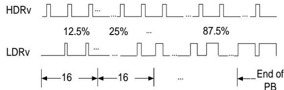
**Figure 12: Pre-Bias startup pulses**
