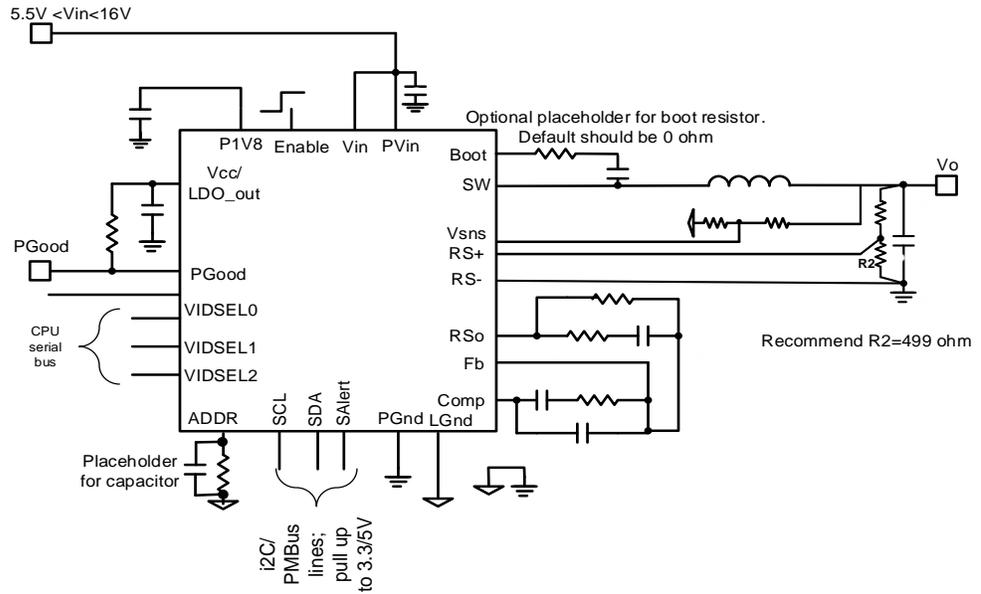
Figure 5: Using the internal LDO,  $V_o > 2.555V$
