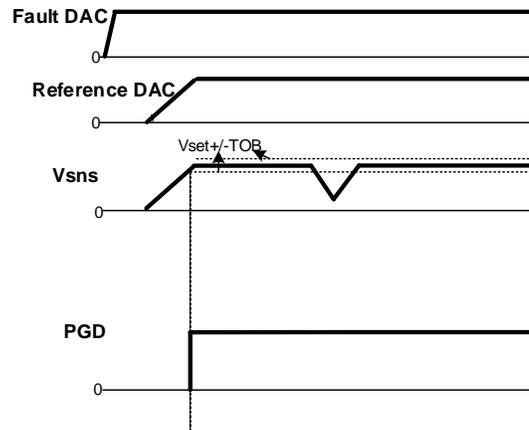
Figure 20: Power Good in PVID mode,  $V_{boot} > 0$  V
