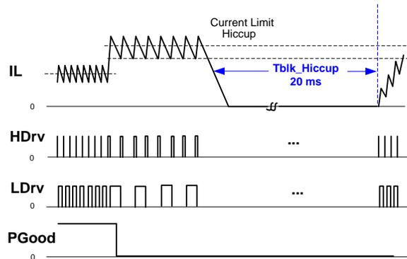
**Figure 14: Timing Diagram for Current Limit Hiccup**
