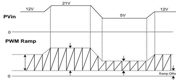
Figure 17: Timing Diagram for Feed-Forward (F.F.) Function
