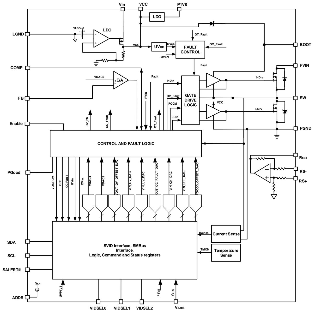
Figure 3: Simplified Block Diagram for IR38263
