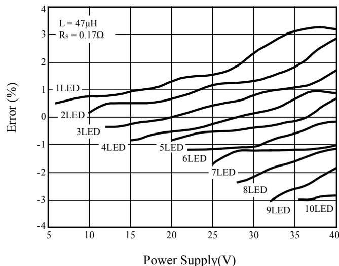
**Figure 3** Output Current Error vs. Power Supply
