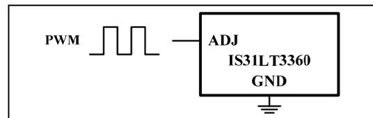
Figure 17 PWM Dimming Control Via ADJ Pin
