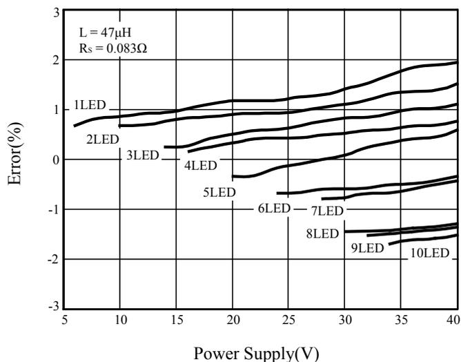
**Figure 2** Output Current Error vs. Power Supply
