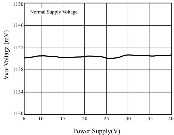
**Figure 9** V<sub>REF</sub> vs. Power Supply (Normal Supply Voltage)
