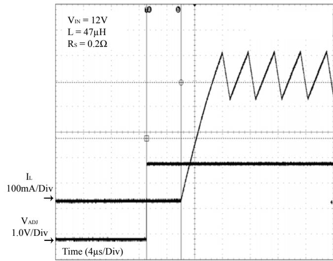
**Figure 13** ADJ Pin Voltage vs. I<sub>L</sub>
