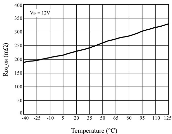
**Figure 12** R<sub>DS\_ON</sub> vs. Temperature
