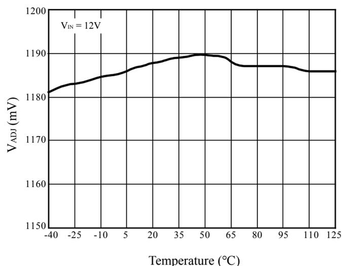
**Figure 11** V<sub>ADJ</sub> vs. Temperature
