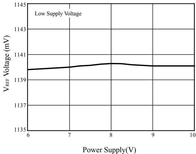
**Figure 8** V<sub>REF</sub> vs. Power Supply (Low Supply Voltage)
