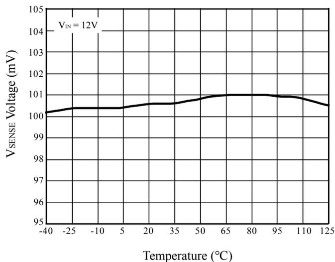
**Figure 10** V<sub>SENSE</sub> vs. Temperature
