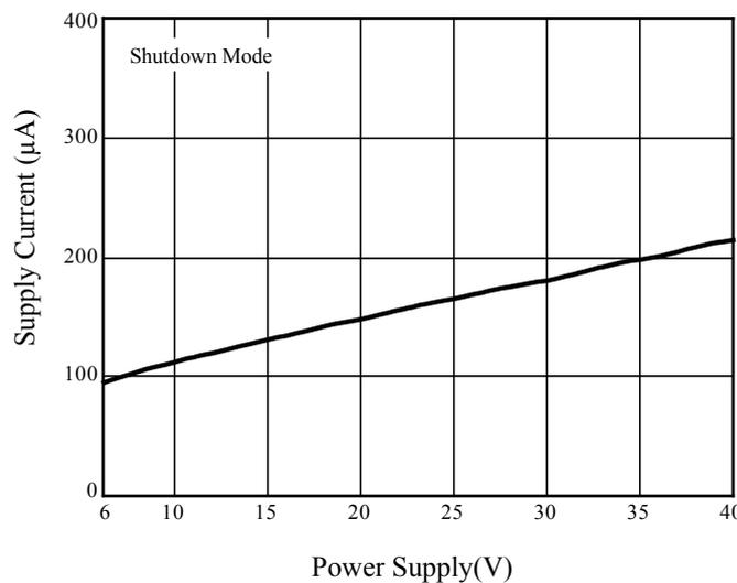
**Figure 7** Supply Current vs. Power Supply (Shutdown Mode)
