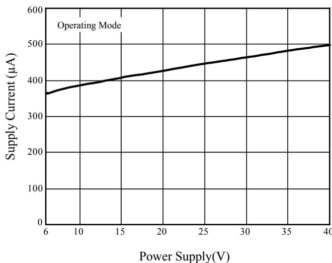
**Figure 6** Supply Current vs. Power Supply (Operating Mode)
