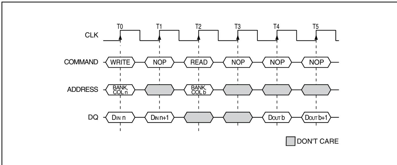
**WRITE to PRECHARGE** ( $t_{WR} = 1 \text{ CLK}$  ( $t_{CK} \geq t_{WR}$ ))
