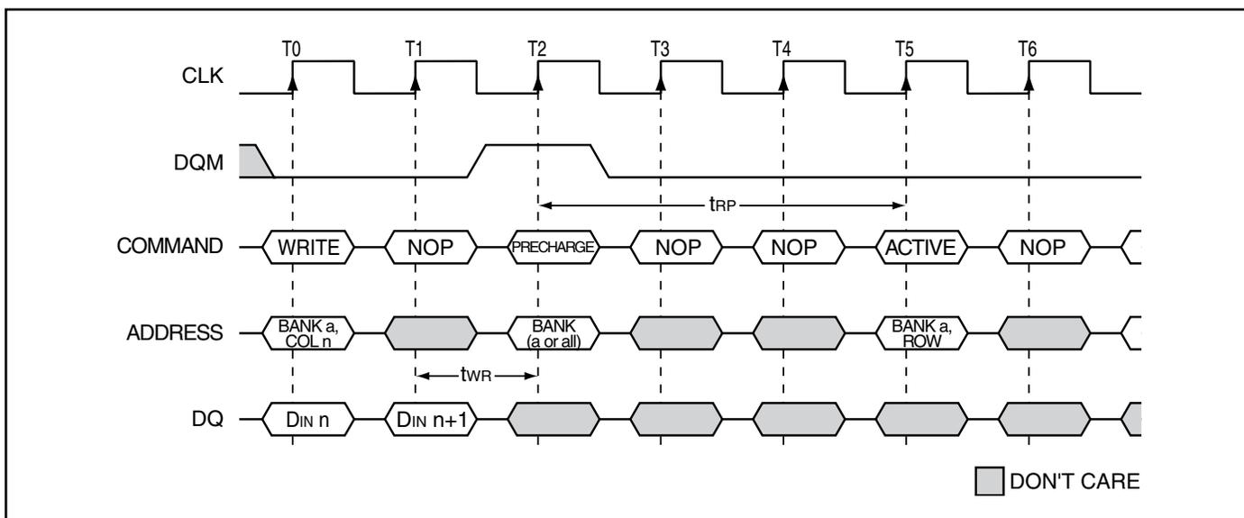
**WRITE to PRECHARGE** ( $t_{WR} = 2 \text{ CLK}$  ( $t_{WR} > t_{CK}$ ))
